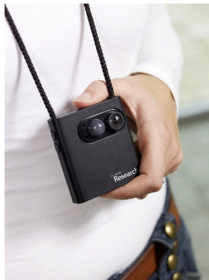
Figure 3-1. The Microsoft SenseCam digital camera. “This wearable device weighs 175 g and passively captures approximately 3,600 first-person point-of-view digital images per typical day” (Kelly et al., 2011b).
