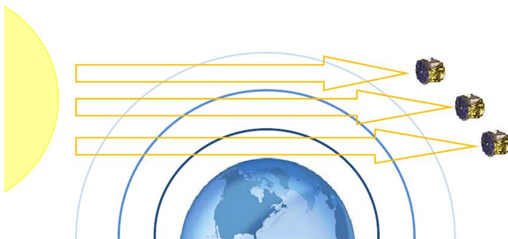
Figure 3.2: Illustration of the ACE profile measurement technique. By scanning layers of the atmosphere at approximately 1 km difference the profile of certain gases can be retrieved.
