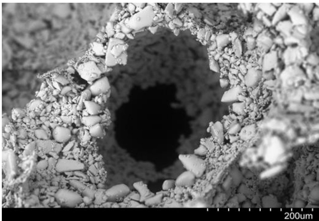
Figure 5.14 - Magnified image of scaffold depicted in Figure 5.13. Some evidence of particle rounding can be seen however, necking is still not evident.
