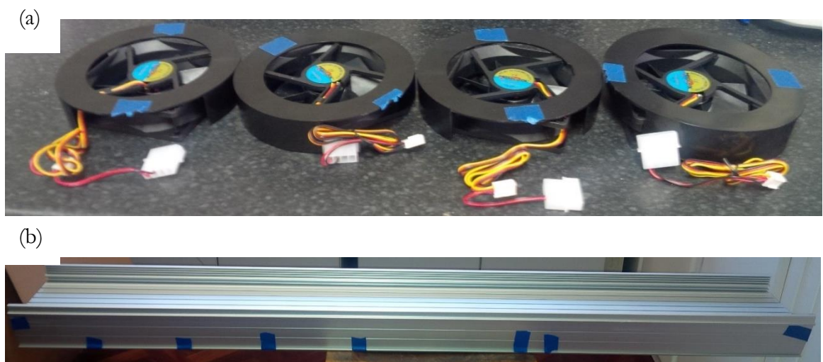
Figure 7.3 (a) The 4 12 V cooling fan for each CREE LED boards for removing heat at intensity values \geq 10\% ; (b) Heat sink for mounting and installing LED's, fans, drivers and for dissipating heats
