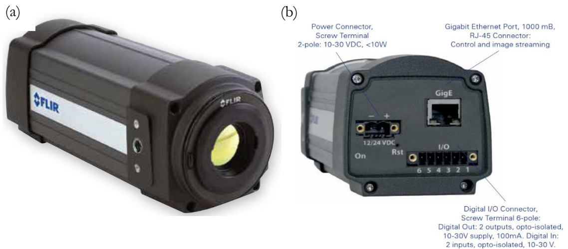
Figure 8.5 FLIR 325sc infrared camera used for acquiring the thermogram, x-y plots and csv data exports; (a) front view of the camera in front and the point of connection to tripod by the side;(b) back view of the showing the power connector screw terminal, Gigabit Ethernet port RJ-45 connector and the digital I/O screw terminal
