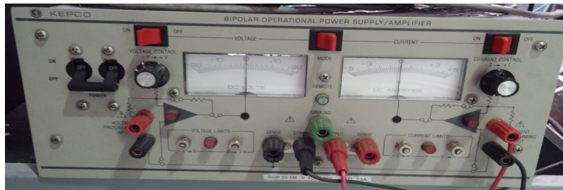
Fig. 4.5 Kepco BOP 20-5M amplifier
