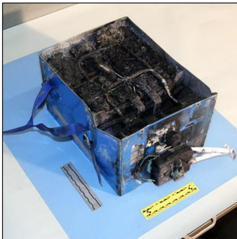
Fig. 1.1 Example of a failed lithium-ion battery in a Boeing 787 Dreamliner [1]
