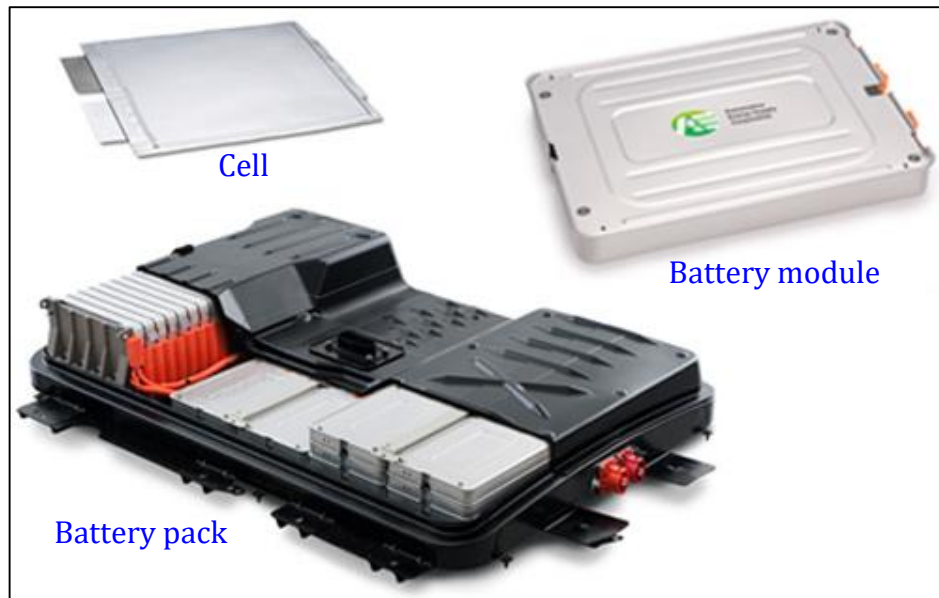
Fig. 2.24 Composition of Nissan Leaf's 24 kWh LMO battery pack [208]
