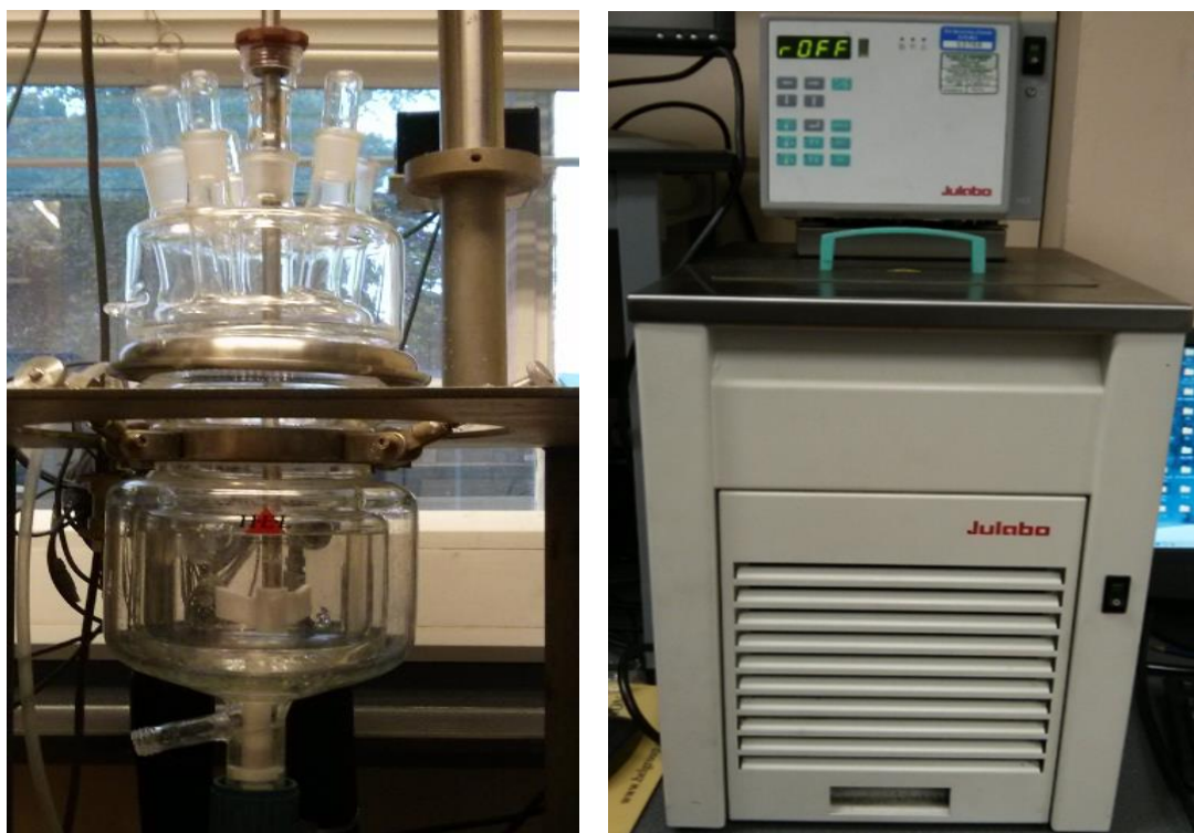
Figure 3.5: Half-litre reactor system (left figure: jacket reactor, right figure: Julabo heating circulator)
