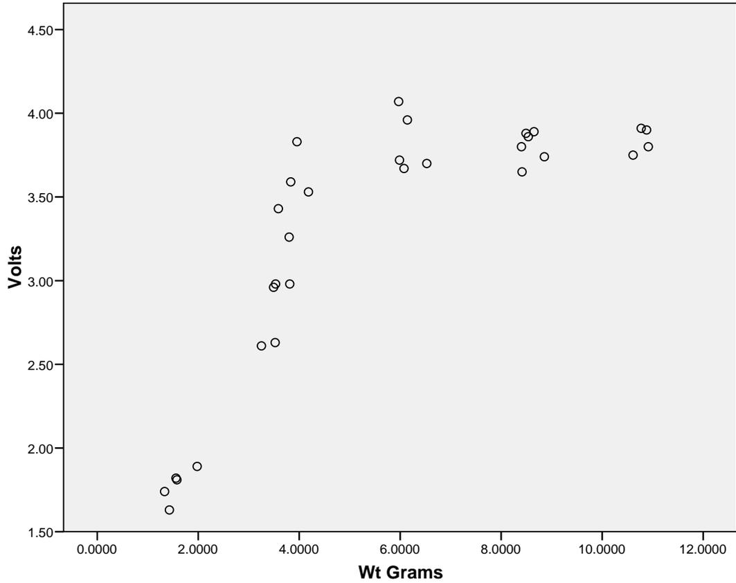
Figure 19 scatter plot of weight versus output of pressure sensor
