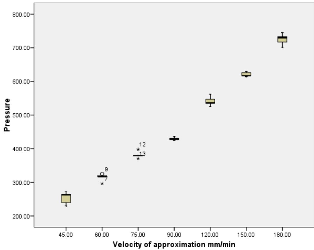
Figure 63 Box plot of results for the medium bodied regular set silicone; velocity against pressure
