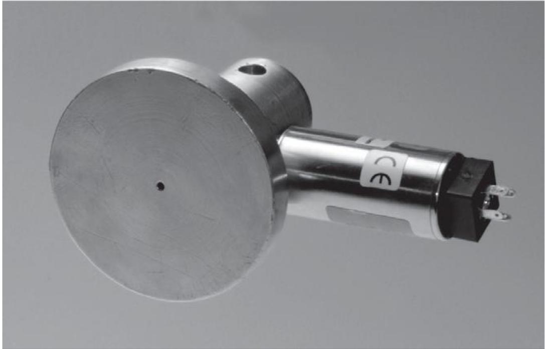
Figure 26 Sensor attached to brass disc with 2mm hole at centre.
