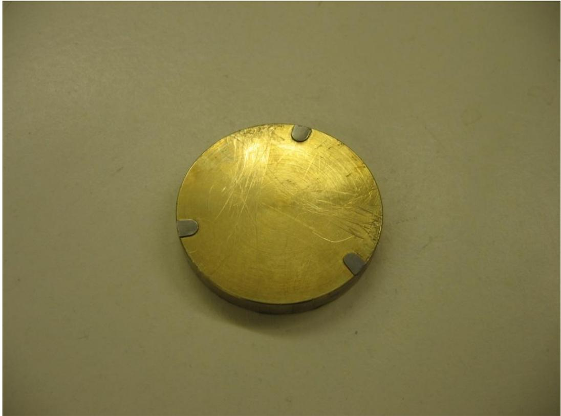
Figure 3 An 'impression tray' used to carry impression material note the stainless steel 'spacers' made from engineers' 'feeler gauges'.
