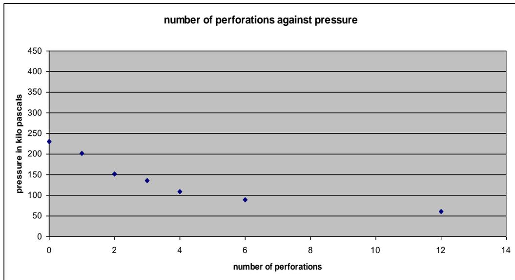
Figure 47 plot of means of results
