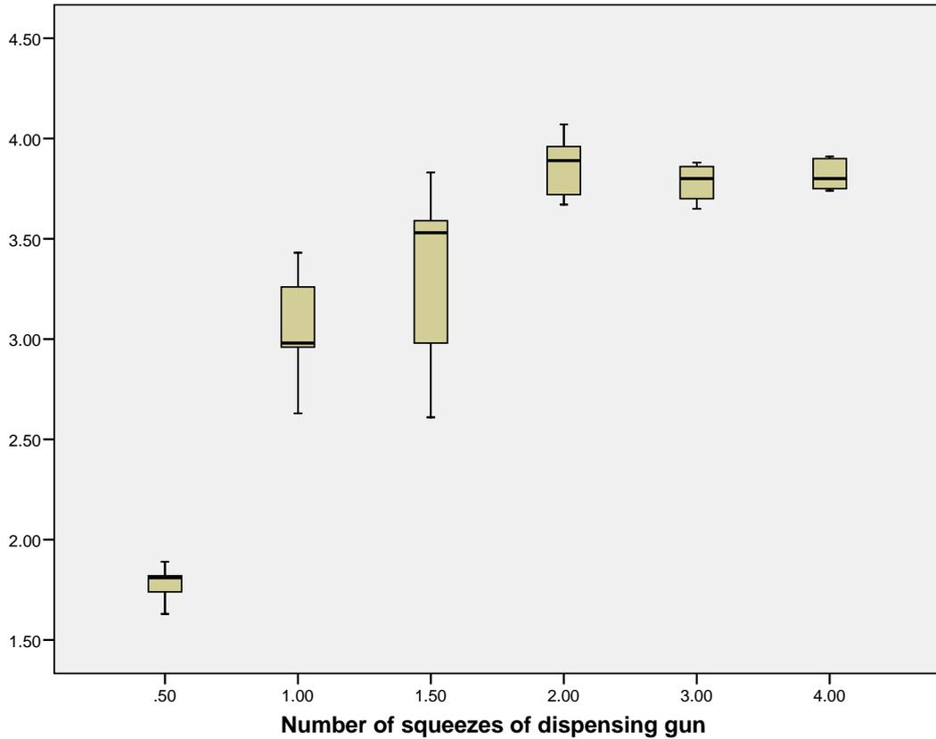
Figure 24 Box and whisker plot of voltage output from the pressure sensor versus number of pull of dispensing gun trigger
