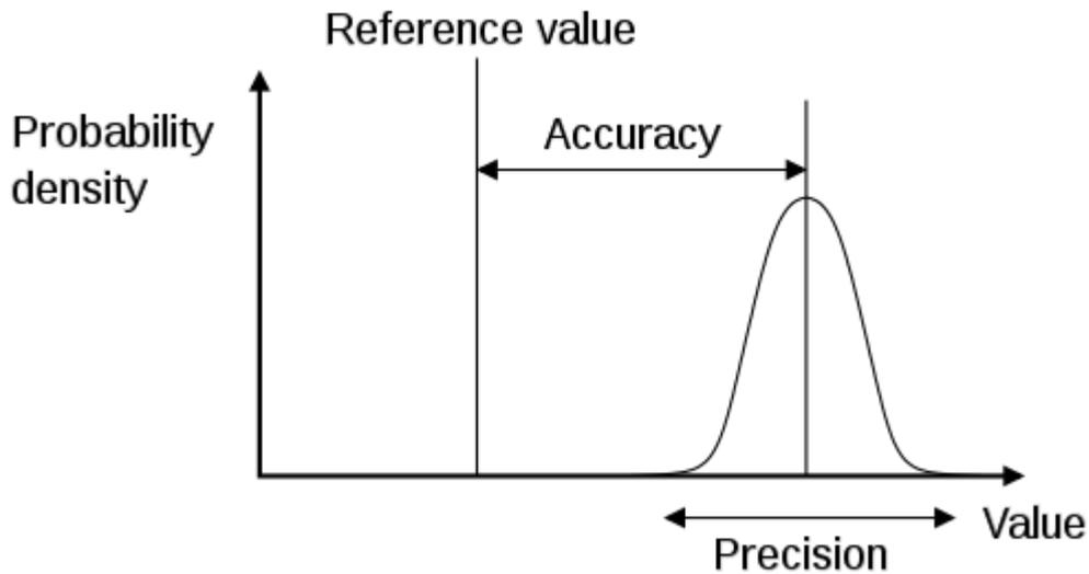
Figure 7 A diagrammatic representation of the definitions of accuracy and precision
