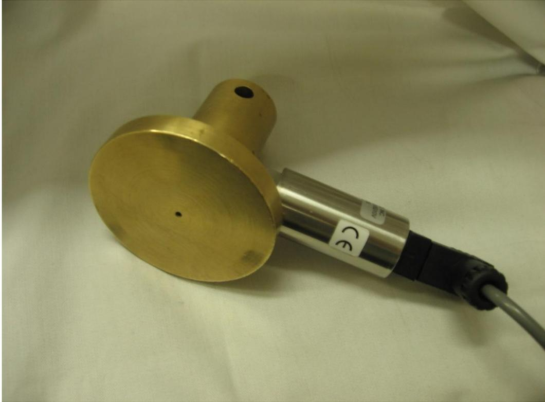
Figure 40 The standard disc with sensor attached
