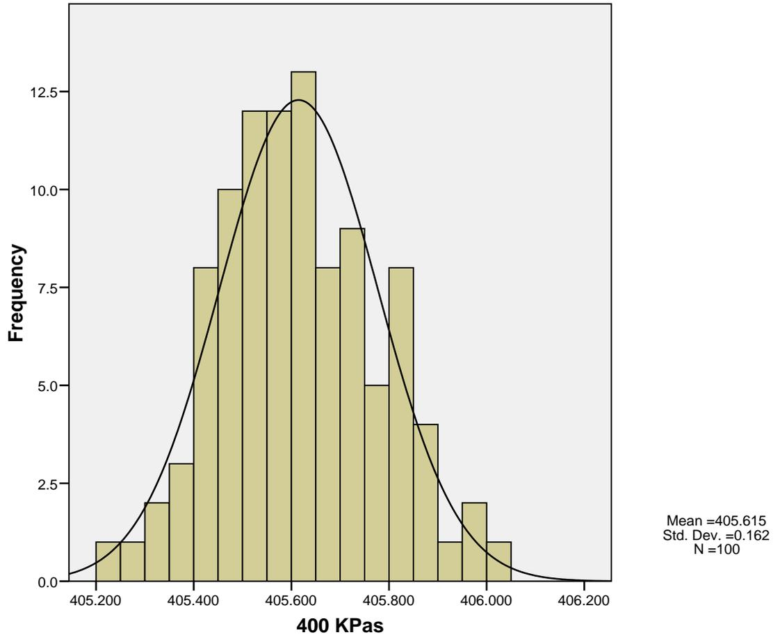
Figure 12 Precision error at a nominal 400KPa; a SPSS legacy histogram of 100 output data with the normal distribution curve superimposed.
