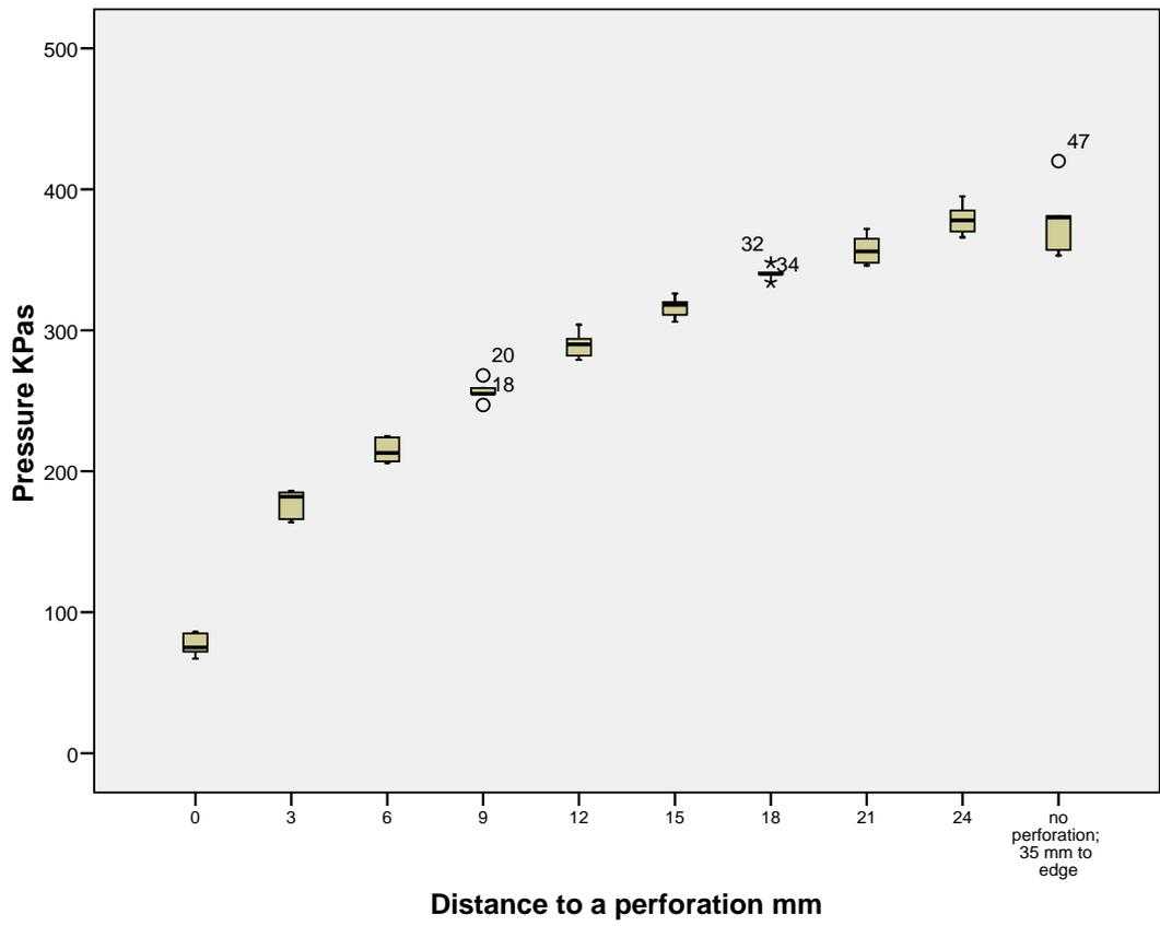
Figure 42 Box plot of results for the 'distance to a perforation' experiment
