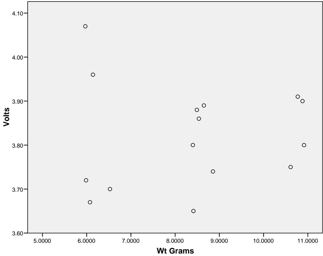
Figure 25 scatter plot of weight versus voltage output from the pressure sensor when more than two squeezes of the trigger of the silicone dispensing gun were used.
