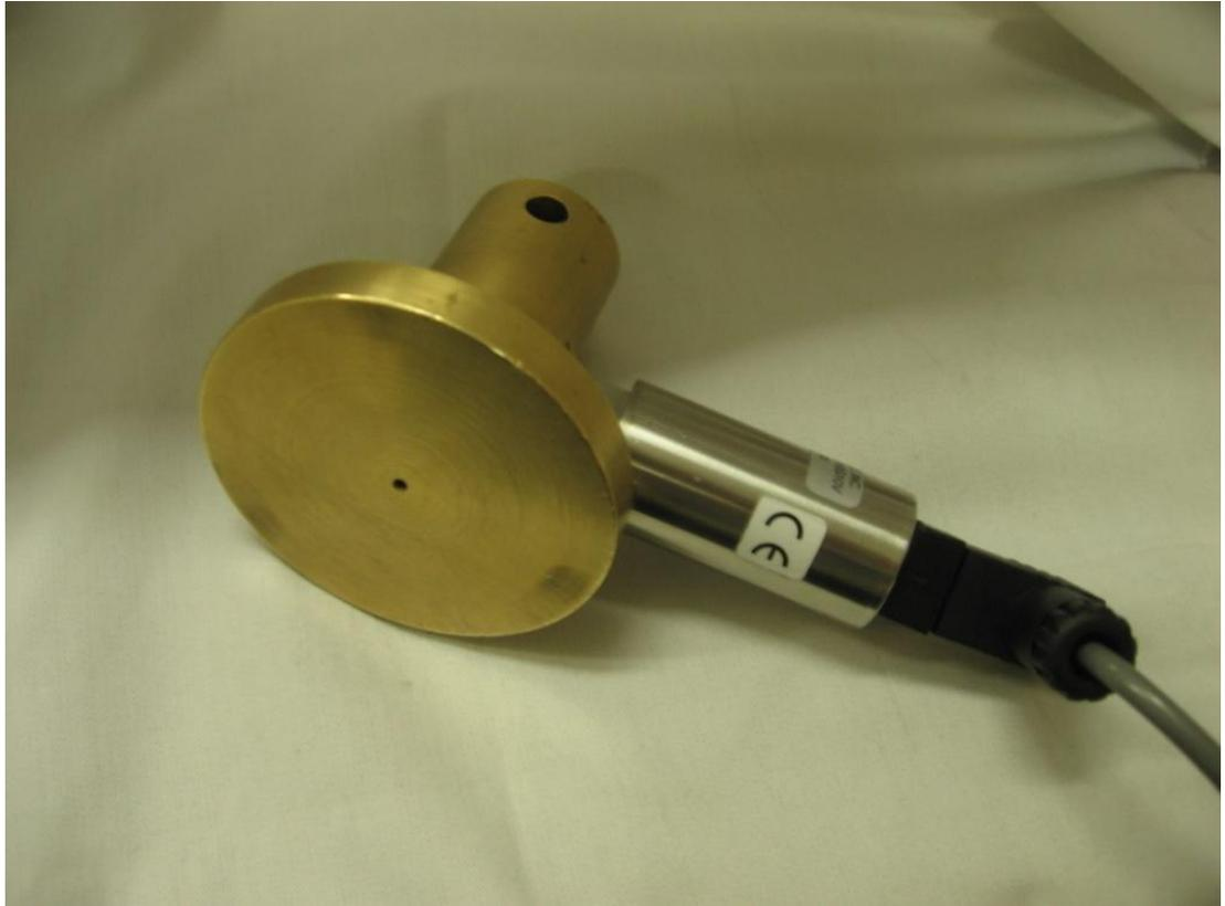
Figure 48 The standard upper disc with sensor attached
