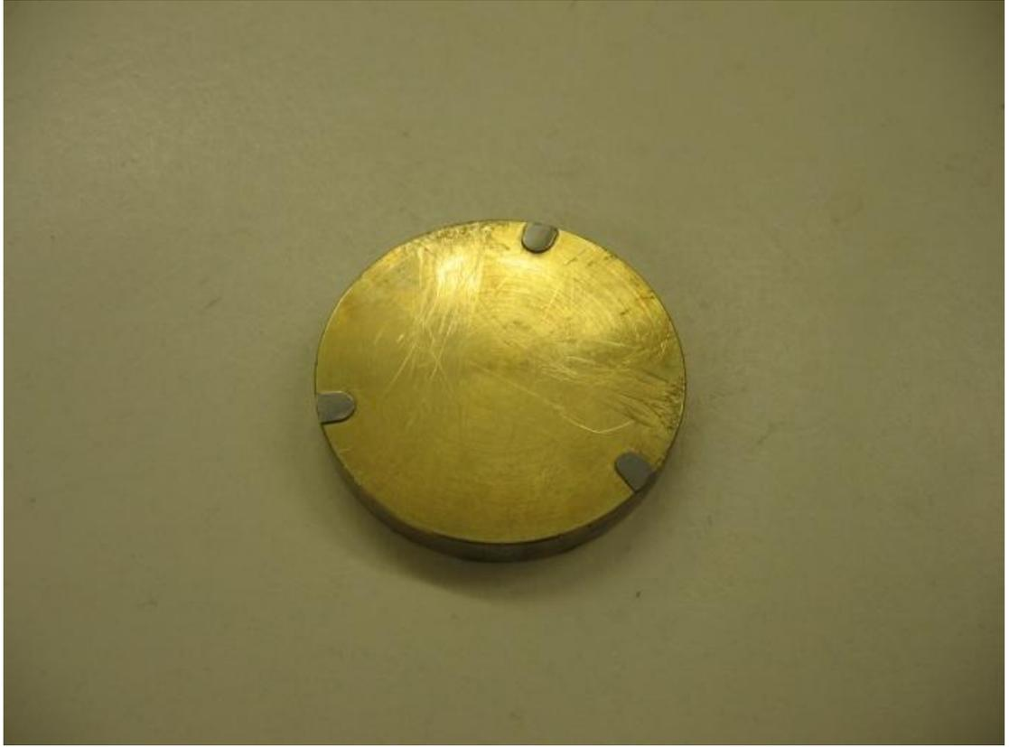
Figure 34 The 'impression tray' for the 'delay' experiment, note the steel spacers.
