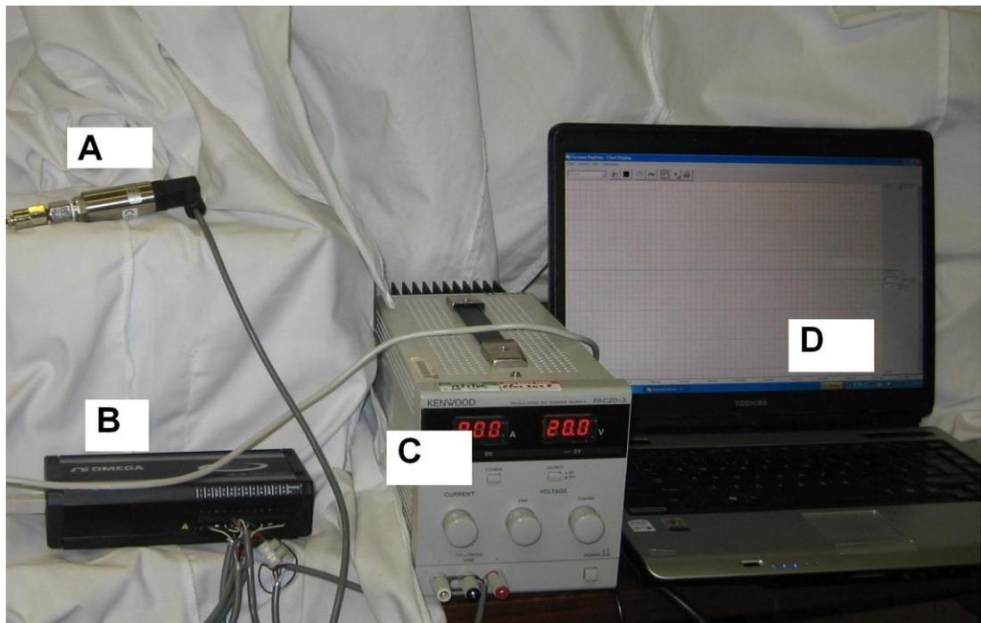
Figure 8 Components of the pressure recording equipment.
