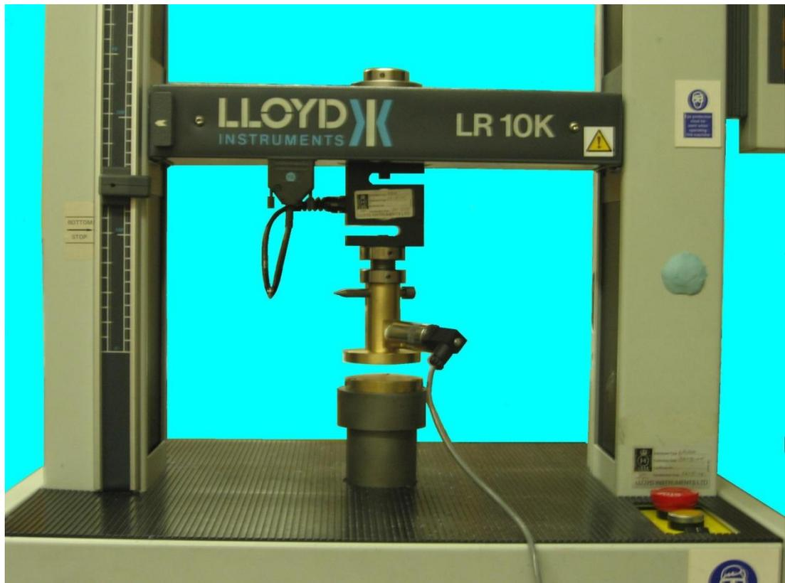
Figure 4 the Lloyd machine with the brass discs mounted
