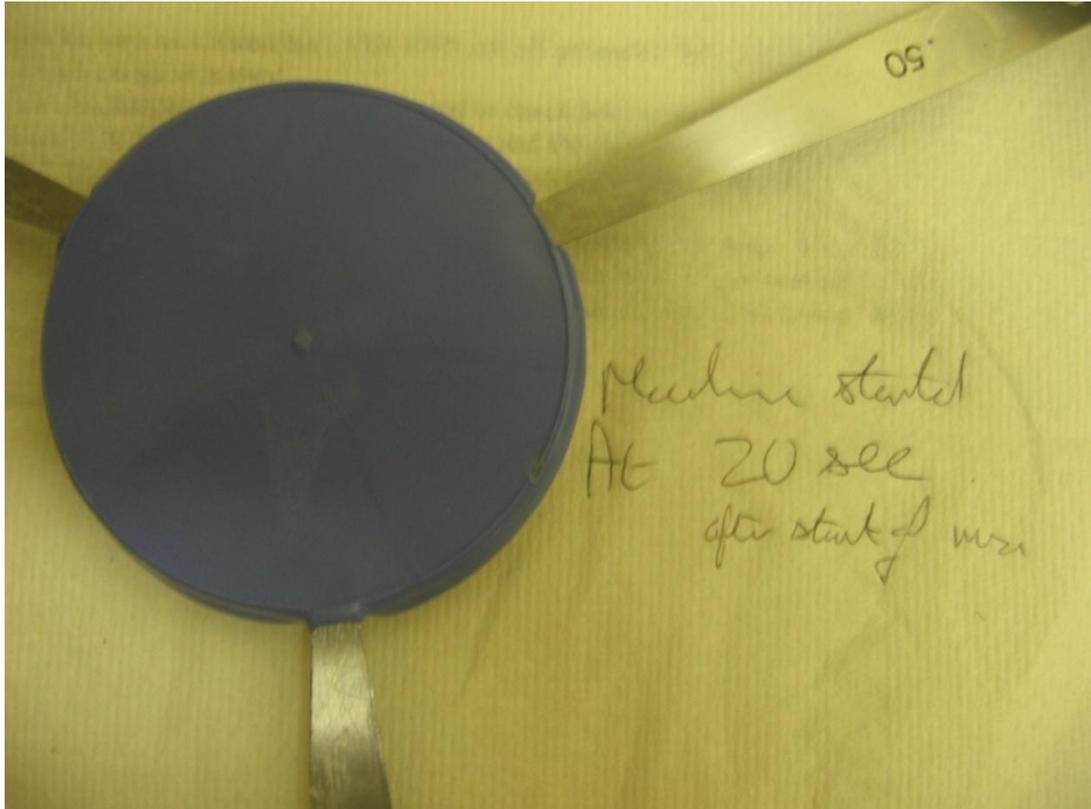
Figure 13 above shows the silicone impression material covering the surface of the steel stops at the end of the experiment.
