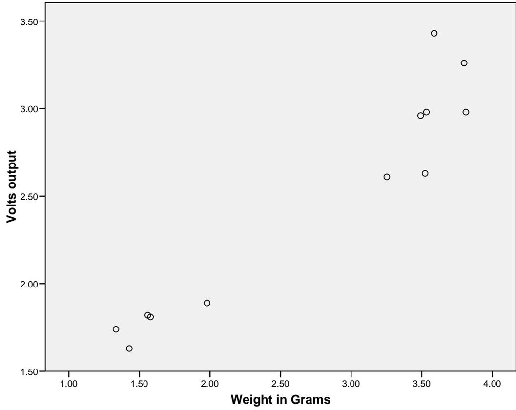
Figure 20 Scatter Plot of weight versus output voltage where there was no overflow of silicone.
