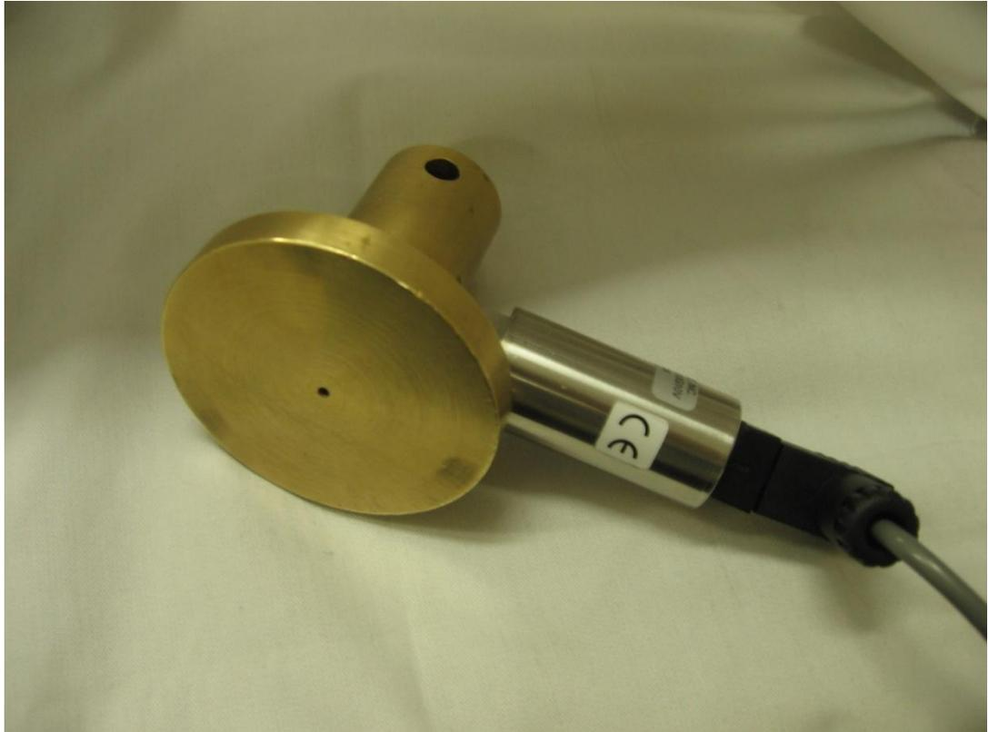
Figure 44 standard impressed disc with sensor attached
