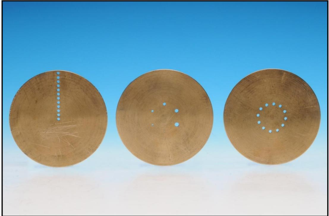
Figure 52 The disc for the distance study is on the left the disc for the size study is in the centre and the number study on the right.
