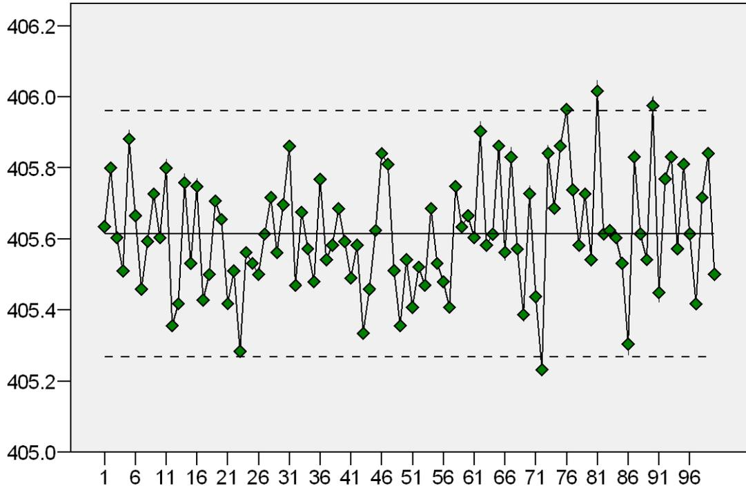
Figure 11 Variation in digital output when sensor held at a nominal 400KPa The bold horizontal line indicate mean and 2Standard deviation from the mean (above and below).
