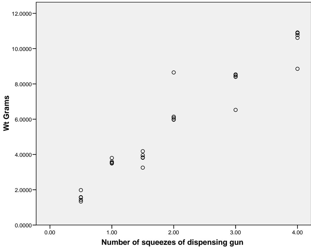
Figure 22 Scatter plot of weight versus number of squeezes on the dispensing gun trigger
