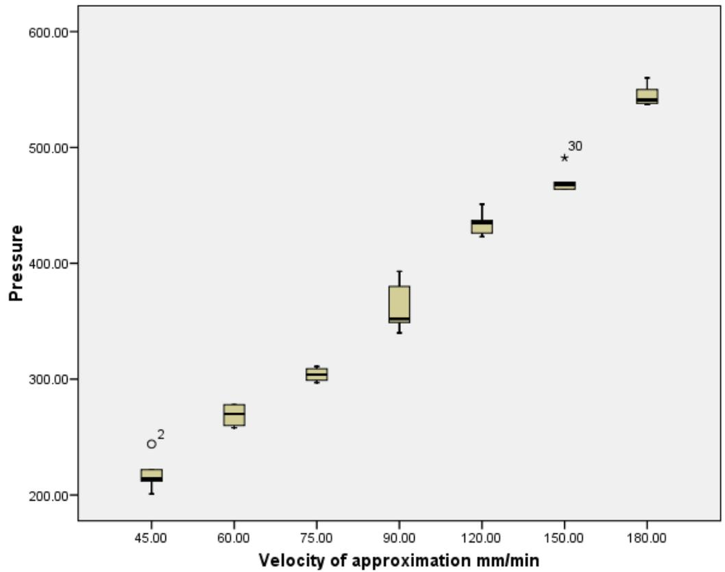
Figure 62 Box plot of results for the light bodied regular set silicone; velocity against pressure
