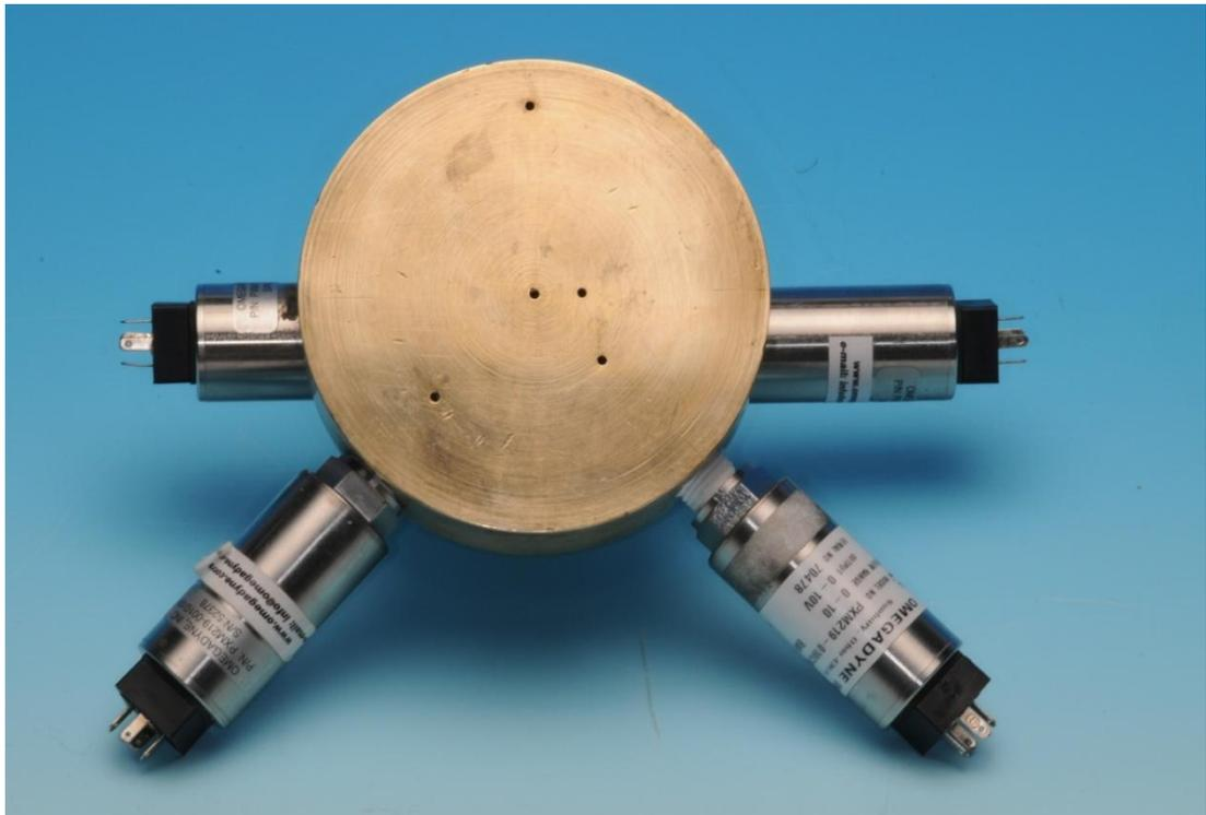
Figure 37 disc used for the experiment to investigate the position of the pressure sensor within the impression
