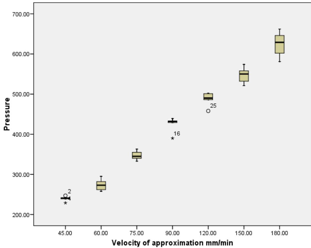
Figure 64 Box plot of results for the light bodied fast set silicone; velocity against pressure
