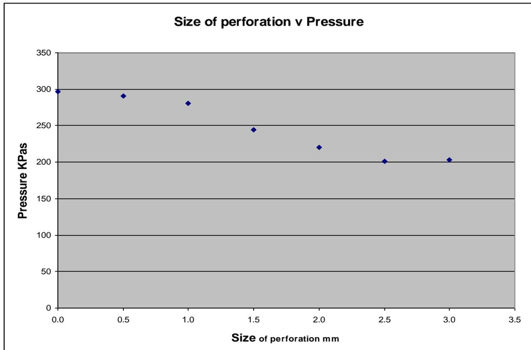
Figure 51 Plot of means of results for the perforation size experiment
