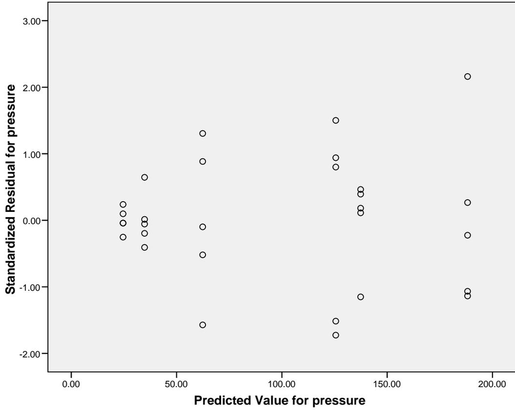
Figure 71 Residuals against predicted pressure using the SPSS factorial ANOVA general linear model (glm) software.
