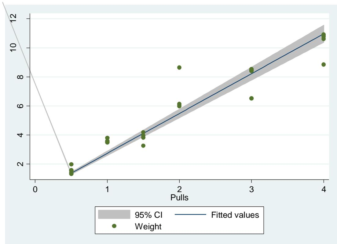
Figure 23 linear regression of weight by the number of squeezes of dispensing gun trigger.
