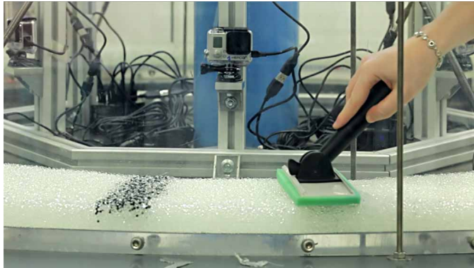
Figure 4.6: Procedure of bed levelling by means of a spongy mop head 200 mm wide.
