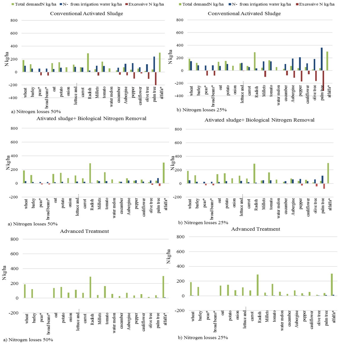
Figure 6-8 The effectiveness of conventional activated sludge, tertiary and advance treatment options under 50% and 25% of nitrogen losses
