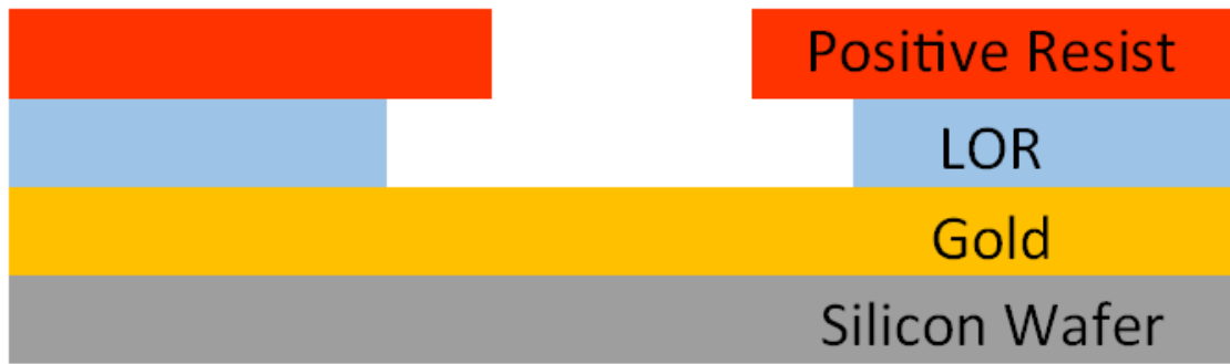
Figure 128: Illustration of the substrate structure after development of the photoresist layers
