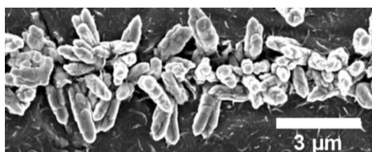
Figure 60: High magnification image of SrCO 3 crystals at a crack on a 16COOH coated substrate
