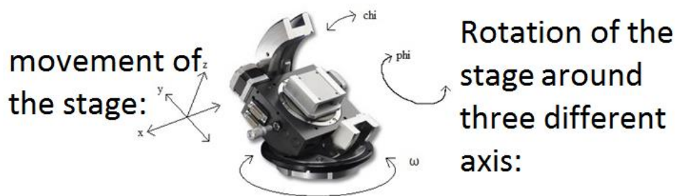
Figure 3.8 Illustration of the movement of the sample stage and rotating angles
