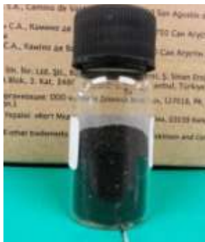
Fig 17 Freshly-synthesised sample of Polyvinylpyrrolidinone-PdNPs ( 46 )
