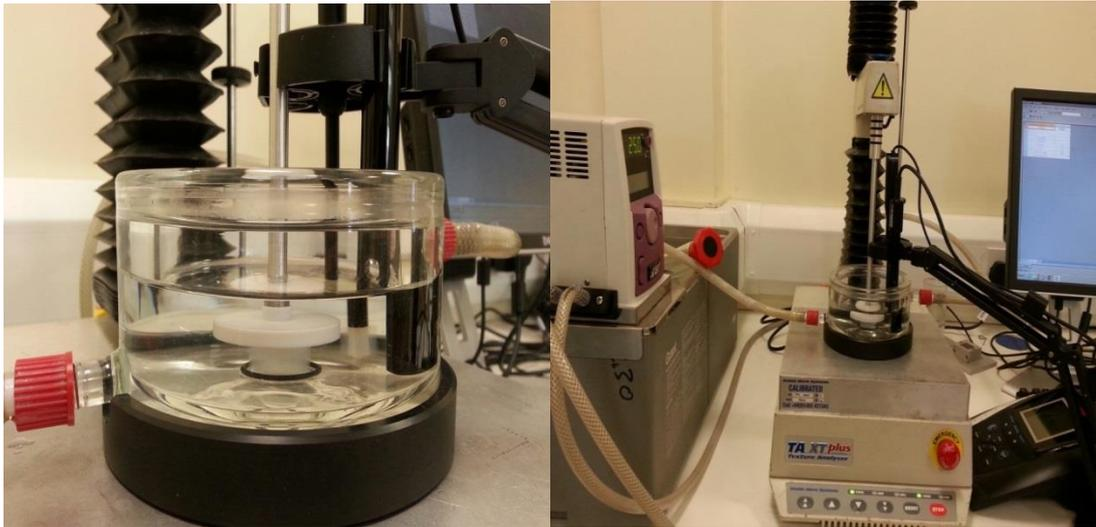
**Figure 3.2** The actual experimental setups attached to the texture analyser.
