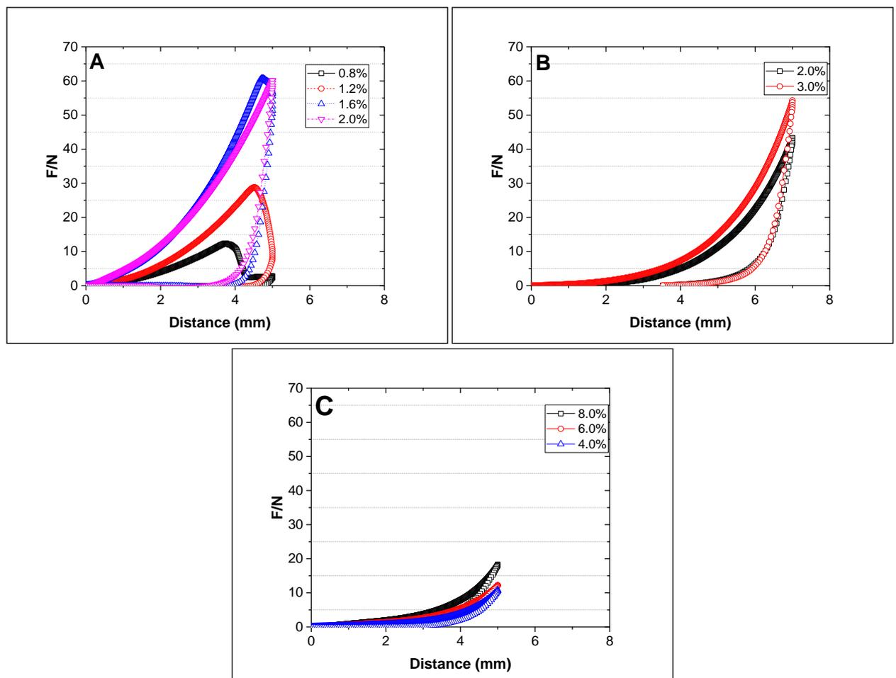
**Figure 4.1** Force (N) against distance (mm) curve for compression of cylinder with the addition for NaCl of  $\kappa$ -c (A), alginate (B) and gelatin (C) gels at different concentration. Tests were performed at a constant rate of 2mm/s to 5 mm distance compression. Alginate compressed at constant rate of 2mm/s to 7 mm distance.
