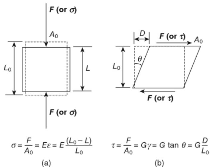
**Figure 2.7** Uniaxial compression (a) and shearing (b) of a sample or product. Uniaxial compression of a sample with original length  $L_0$  and area  $A_0$  and the Young's modulus  $E$ . (b) Shear stress  $\tau$  acting on opposite planes causing the distortion of the specimen with the shear modulus  $G$  and the area of  $A_0$ . Adapted from (Lu 2013).
