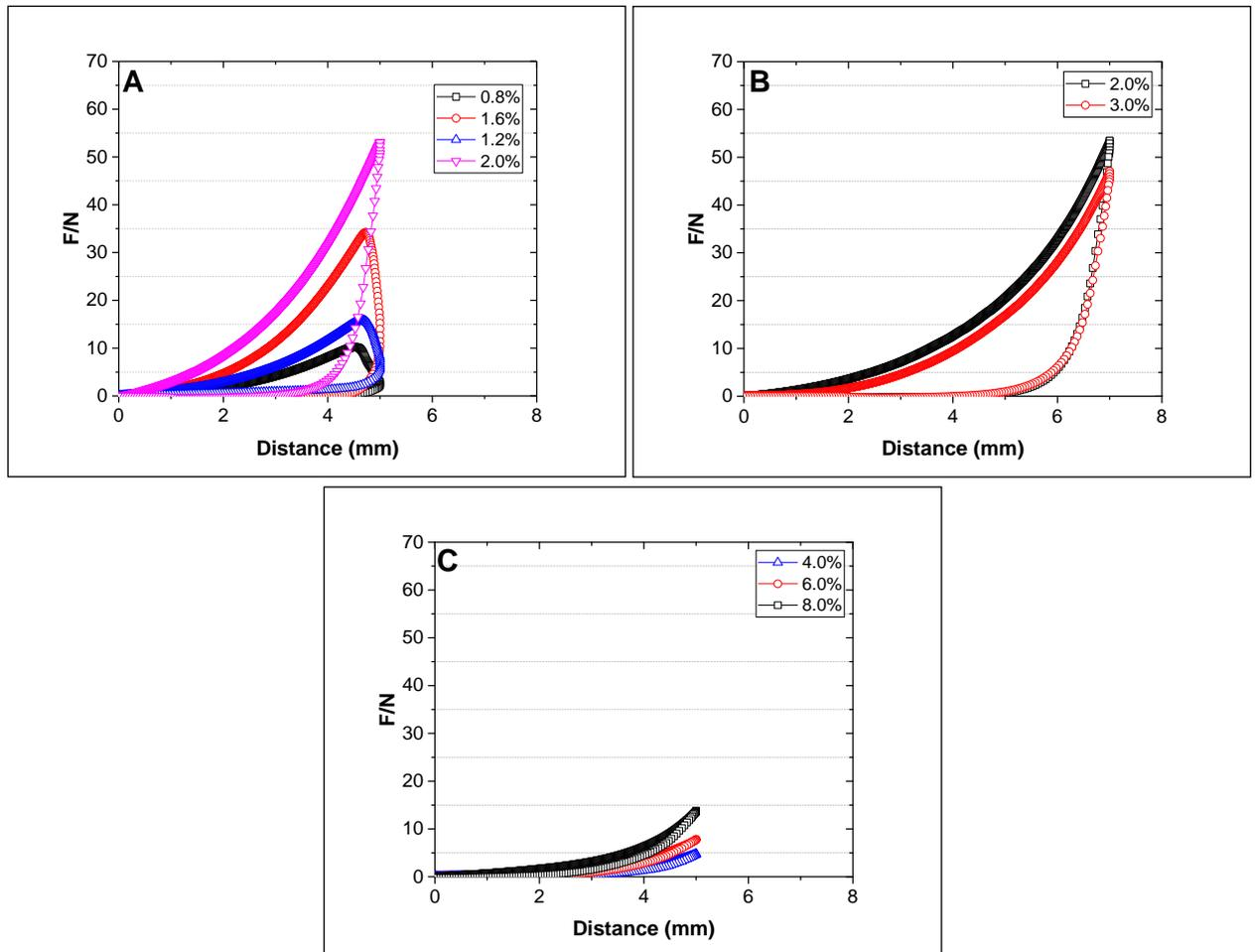
**Figure 4.2** Compression fracture force (N) against distance (mm) curve for compression of cylinder with the addition for glucose of  $\kappa$ -C (A), alginate (B) and gelatin (C) gels at different concentration. Tests were performed at a constant rate of 2mm/s to 5 mm distance compression. Alginate compressed at constant rate of 2mm/s to 7 mm distance.
