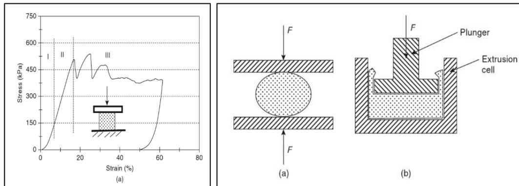
**Figure 2.8.** Example of Stress-strain (or  $F$ - $D$ ) curves of cylindrical apples tissue specimen under uniaxial compression. The stress-strain curves are approximately categorize into three phases of deformation: elastic, yielding and post yielding. Two types of compression test: (a) the uniaxial compression test between plates and (b) the simple compression-back extrusion test. Adapted from (Lu 2013)
