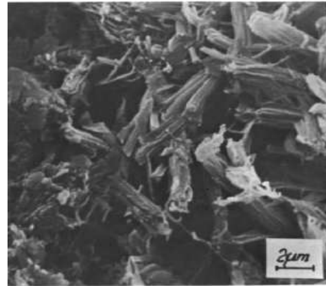
Figure 2-11 Secondary electron image of a tobermorite 11-A after carbonation 30 days at 10%CO 2 and 75%RH [247]
