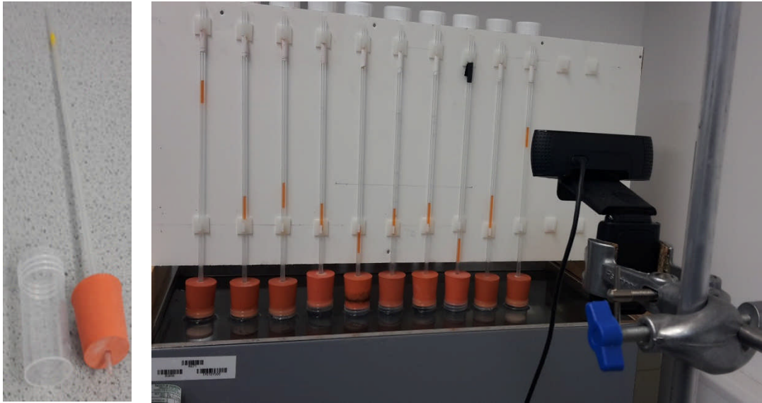
Figure 3-9 Accessories and setup for recording the chemical shrinkage of cements
