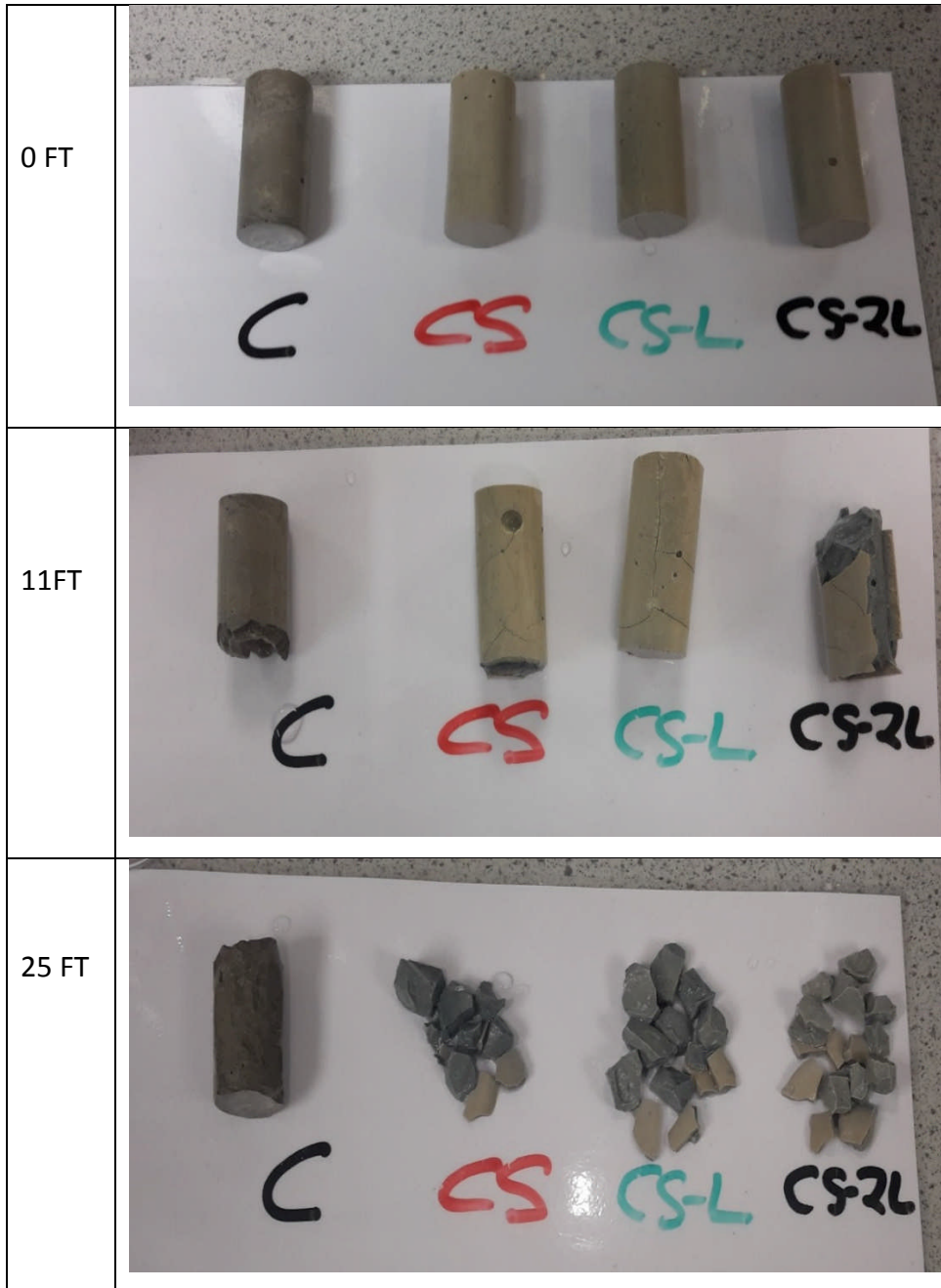
Figure 6-15 Effect of cement composition on freeze-thaw: Cement pastes observations.
