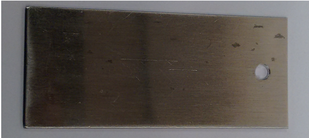
Figure 5.1: Aluminium wedge used to drive dissection, the rounded edge can be seen in the left of the image.
