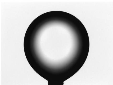
**Figure 6-5 The reversed pendant drop of dodecane in water phase.**
