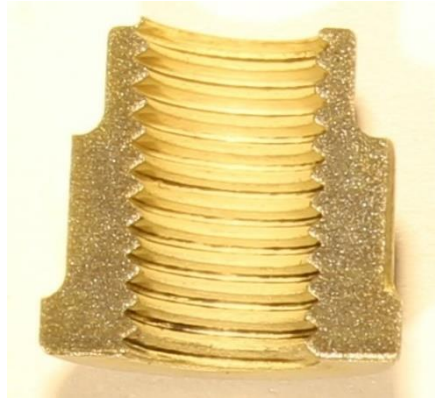
Figure 6.26: Silver Coating Condition (Sample 3A)
