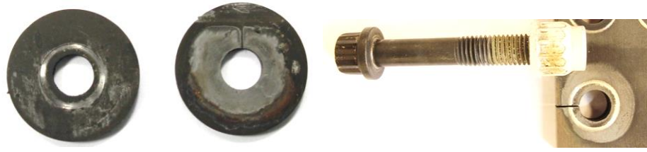
Figure 3.20: a) Typical Washer-Joint Interface, b) Silver Transfer Post-Ageing
