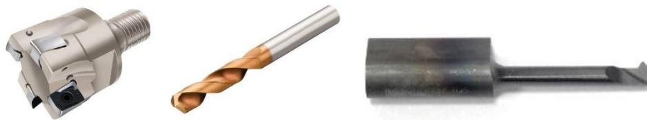
Figure 6.15: Cutting Tools: a) Walker shoulder mill F4041, b) Solid Carbide Drill 5.5 mm, c) Supermini Type 105
