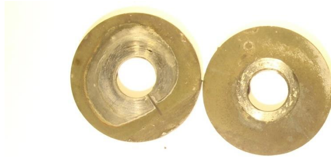
Figure 5.12: Seizure in the bearing Surfaces
