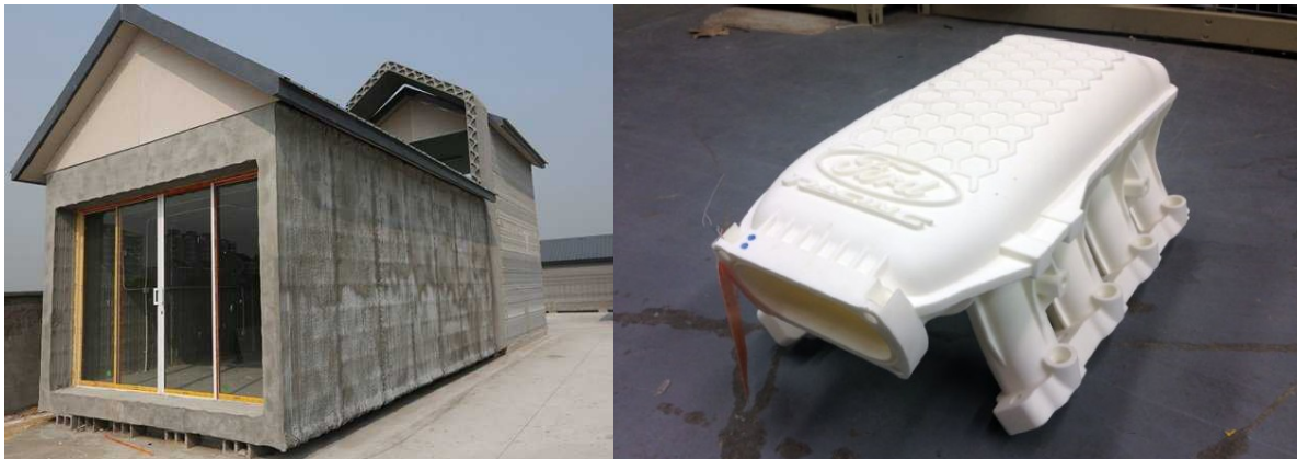
Figure 1.17 - Two examples of items made using AM from the engineering industry. A concrete printed house [34] (left) and a printed car engine part by Ford [35]
