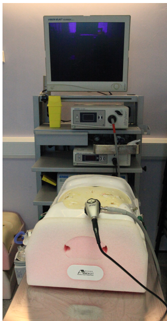
Figure 1-5: An example of a Laparoscopic Stack system. A box-trainer can be seen in the foreground with a laparoscopic camera. On the shelving unit in the background the display monitor and light source are seen.
