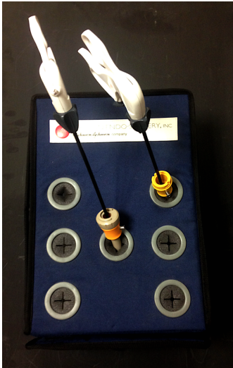
Figure 1-4: An Ethicon™ laparoscopic box trainer with 6 port-sites and two laparoscopic instruments in-situ.
