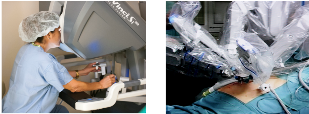
Figure 1-3: RAS Set up: The da Vinci System®; the operator sits in a 'booth' and controls the robotic arms remotely using his/her hands and feet. The robotic 'arms' (seen here on the right) are introduced in a similar manner to ports/instruments during laparoscopic surgery
