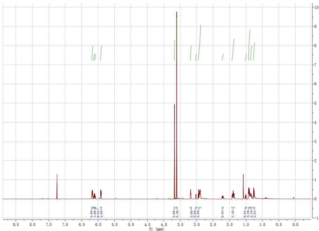
Figure 3.7: ^1\text{H} NMR spectrum of the product from the Diels-Alder reaction in hexane.
