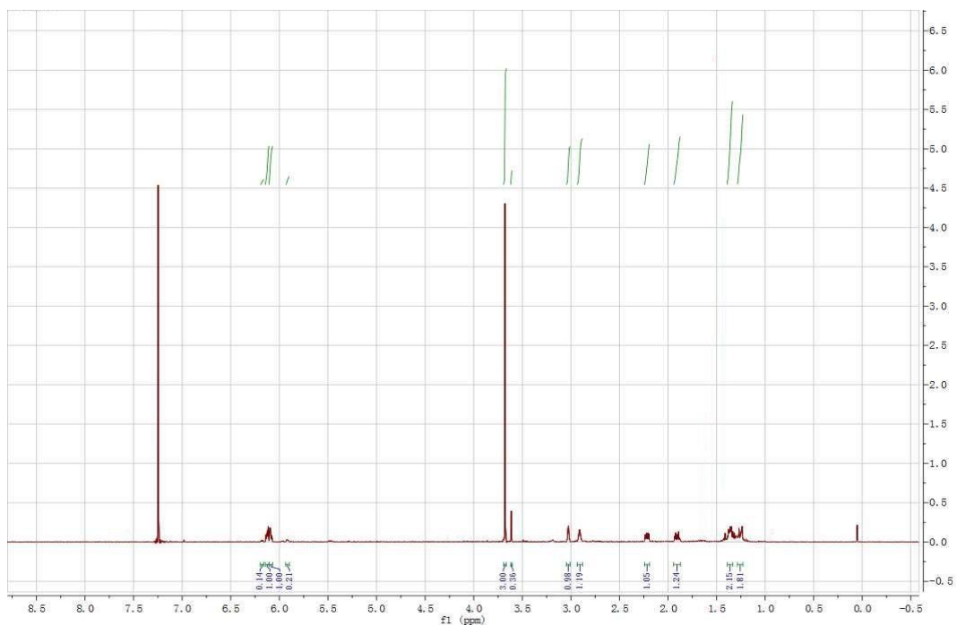
Figure 3.8: ^1\text{H} NMR spectrum of the 83.3% exo product after separation from the Diels-Alder reaction in hexane.
