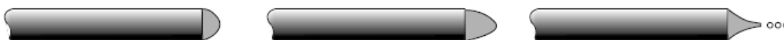
Figure 2.3: The shape of drops at the capillary tip while producing spray adapted from [96].
