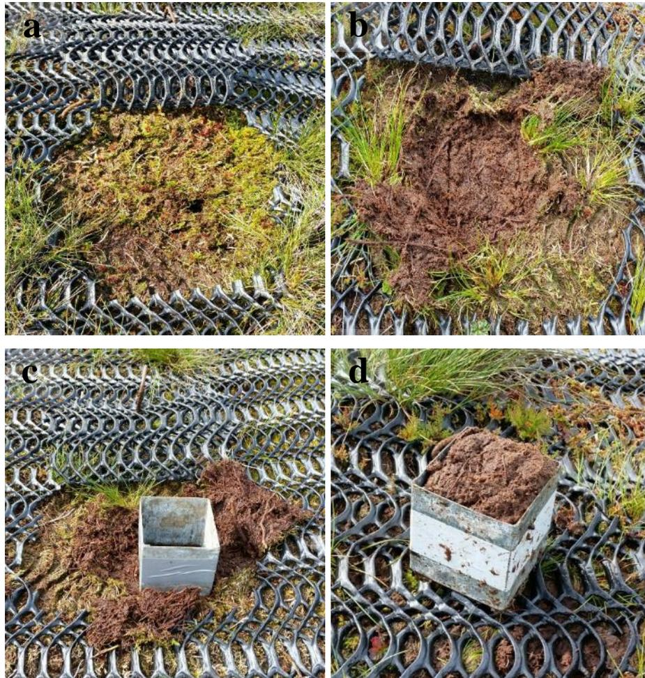
**Figure 5.4 a-d** Collection of after samples for Laboratory *K* analysis using the modified cube method; a) track cut away to expose vegetation, b) clearing of vegetation to reveal peat surface, c) locating of metal box and start of sample extraction, d) sample after extraction.
