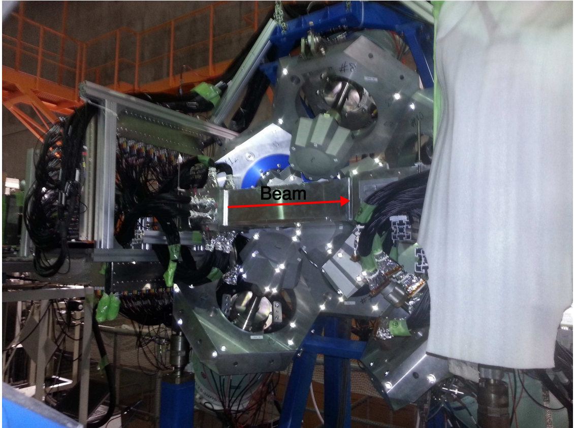
Figure 3.5: A photograph of the set-up of the F11 focal plane for RIBF97. EURICA and the chamber with the active stopper WAS3ABi.
