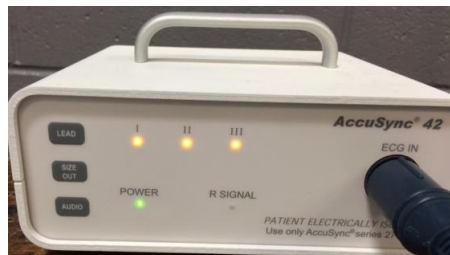
FIGURE 3.10: Shows the new ECG used for triggering data (for high and/or low voltages), manufactured by Accusync.
