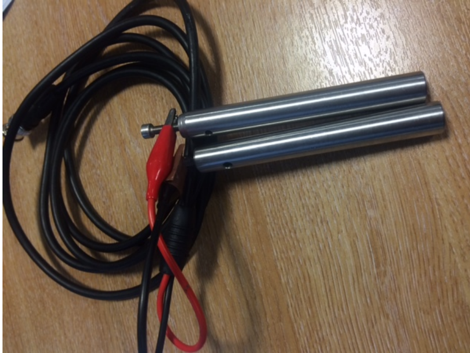
FIGURE 3.3: Shows the bars we used as an electrocardiogram.
