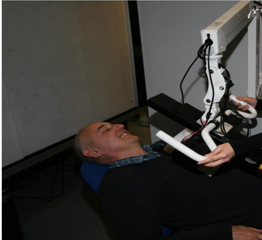
FIGURE 3.4: Four-channel MCG. It is placed as close as possible to the chest.
