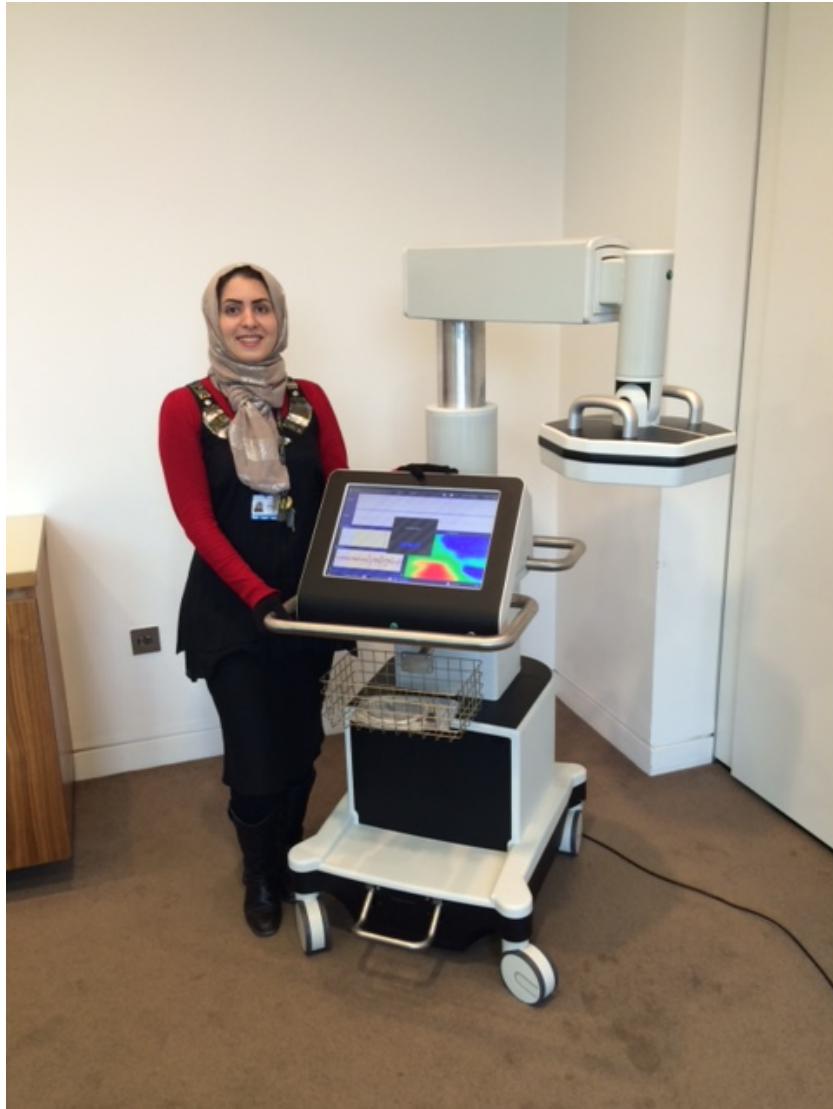
FIGURE 7.1: Shows MCG alpha-plus device, including 37 small coils with the portability feature.
