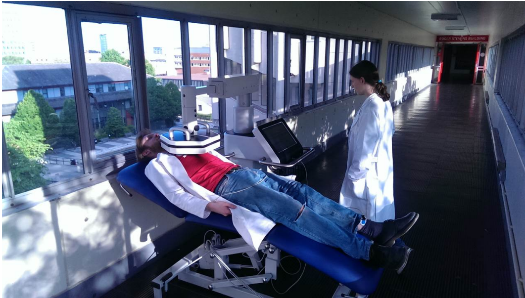
FIGURE 7.2: Shows the portable MCG alpha-plus, recording an MCG scan at the university of Leeds.
