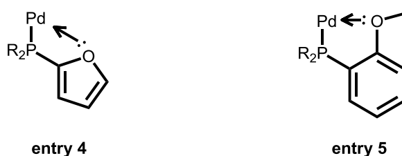
Figure 53. Hypothesised bidentate binding modes of P(2-Furyl) 3 (Entry 4) and P(2-MeOC 6 H 4 ) 3 (Entry 5) ligands coordinated to Pd metal centres.
