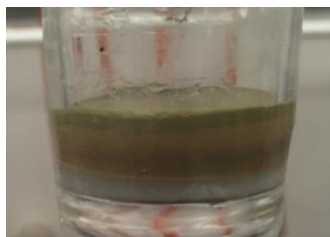
Figure 48. Photograph of the Celite®-pad after hot-filtration of the reaction shown in Scheme 52 . The green solid collected at the top was identified as \text{Ag}_2\text{CO}_3 based on the appearance.
