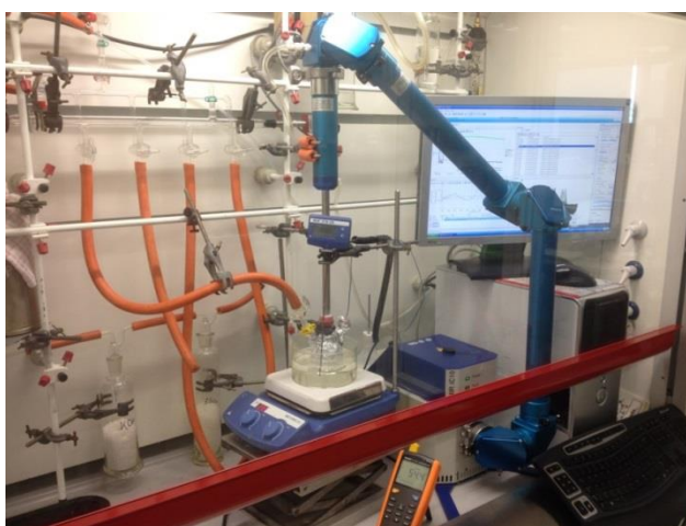
Figure 12. Experimental set-up for following the kinetics of the reaction shown in Scheme 39 using the ReactIR TM , an in situ FT-IR instrument.
