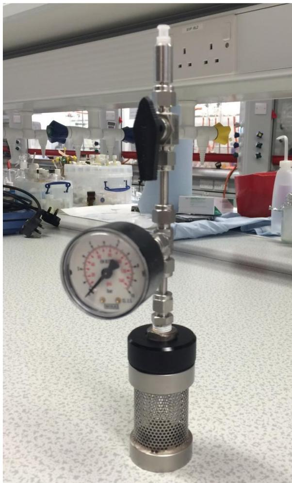
**Figure 38:** Photograph of a 10 ml gas-tight Fisher-Porter vessel equipped with a pressure gauge and a Luer lock adapter.
