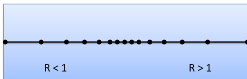
Figure 3.8. The typical nodal distribution for a double geometric grid in DICTRA where R is the geometrical factor.
