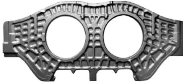
Figure 2.6. F-22 bulkhead forging. Approx. 3000 kg, 1.7 m high by 4 m wide [45].
