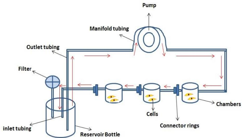
Figure 2.2: Schematic diagram of Quasi-vivo® set up. Red arrows indicate direction of medium flow. Black arrows indicate parts of the set up.
