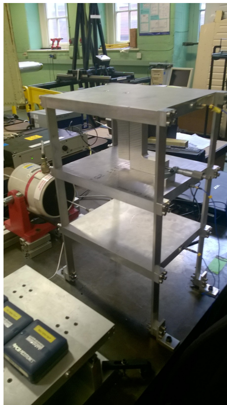
Figure 6.23: Experimental 3-DOFs Rig with nonlinear element in place
