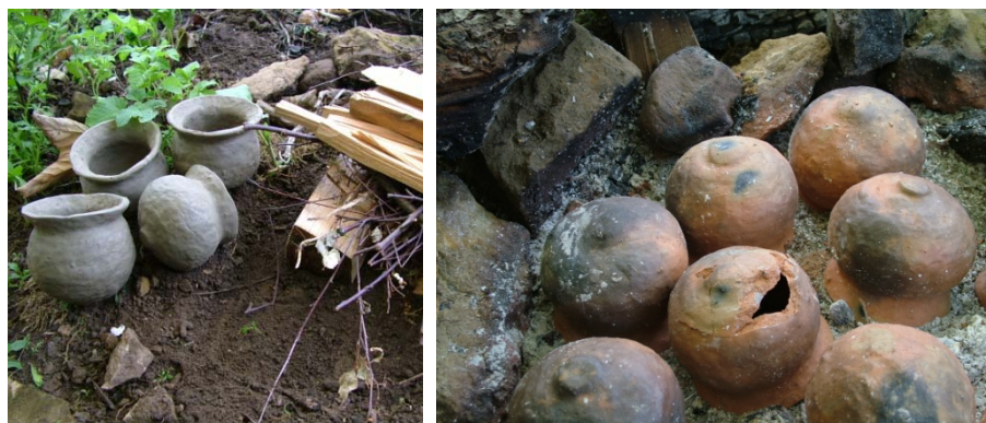
Figure 7. 15. Pre-fired clay is grey but transforms to an oxidised red with firing. The process of construction embodies a management of material transformation.
