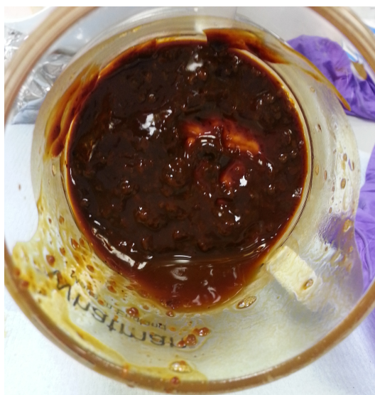
Fig. 6.32 Ferrihydrite precipitation - pH 1.5 in the absence of sulphate ions and air/oxygen bubbling
