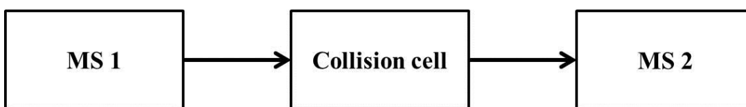
Figure 1.15: Typical arrangement of an in-space tandem mass spectrometer
