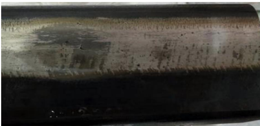
Figure 3-5 Rail surface after application of nital etch
