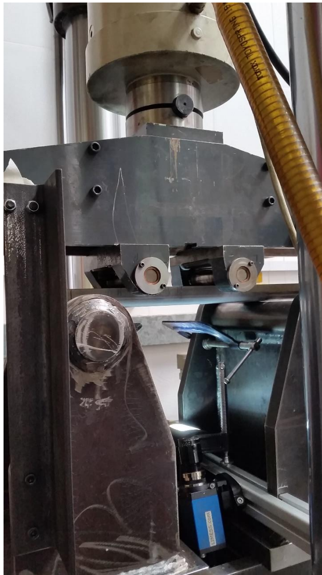
Figure 6-9 Four point bending test with application of DIC
