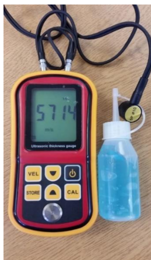
Figure 6-3 GM100 ultrasonic thickness gauge couple with 10mm diameter transducer. Working frequency 5MHz, accuracy \pm 1\% , and thickness measuring range of 1.2-225mm (steel).
