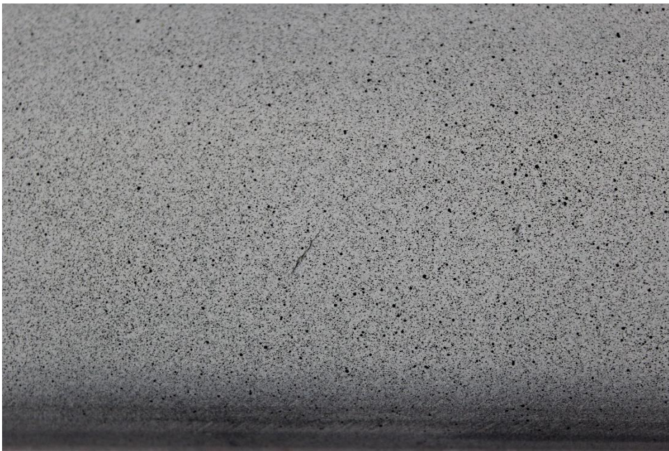
Figure 6-7 Random speckles pattern created on Sample A
