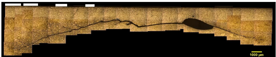
Figure 3-8 Etched longitudinal cross section for sample A. White dash near surface represent location of white etching layer
