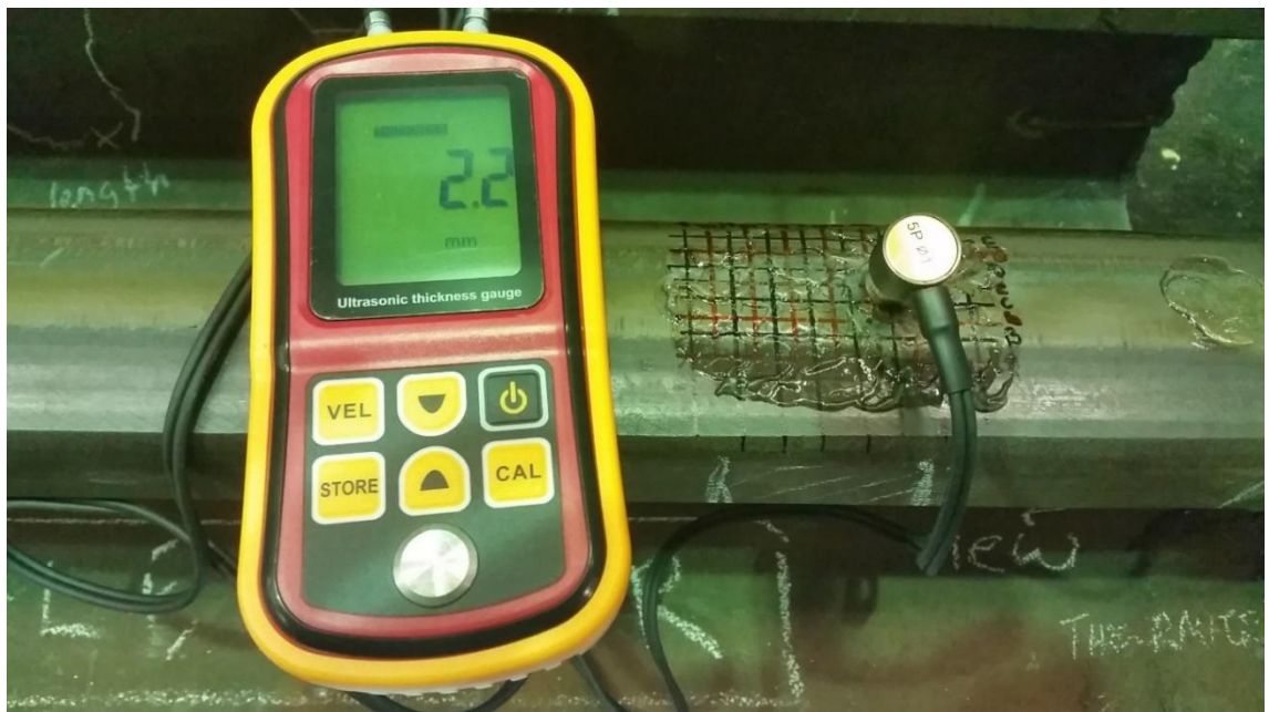
Figure 6-5 Internal defect was identified on Sample 1 with a depth of 2.2mm from the rail surface.
