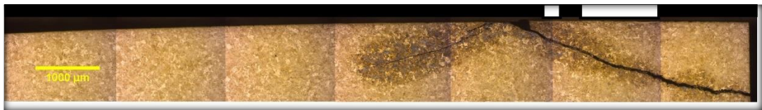
Figure 3-14 Close up on surface crack observed on sample B2. White dash near surface represents the location of white etching layer.
