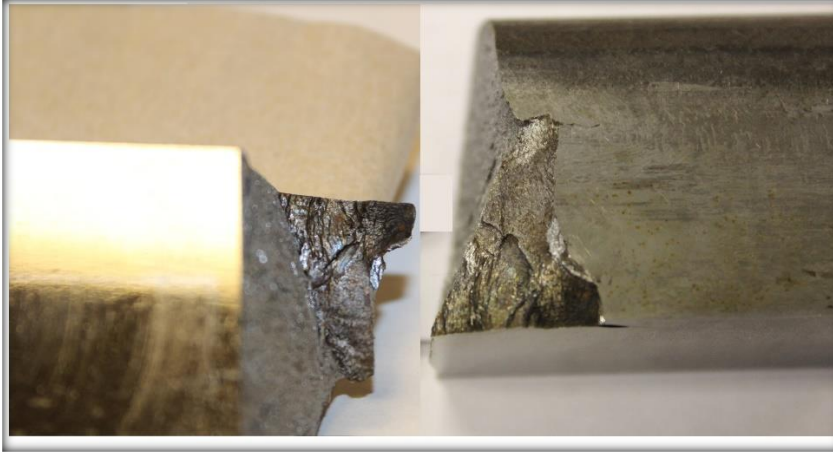
Figure 3-17 Crack faces lying underneath the surface of the broken sample A
