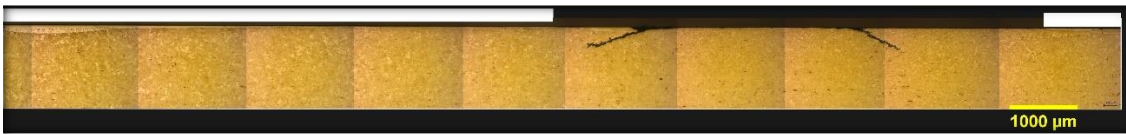
Figure 3-10 Etched longitudinal cross section for sample C. White dash near surface represent location of white etching layer
