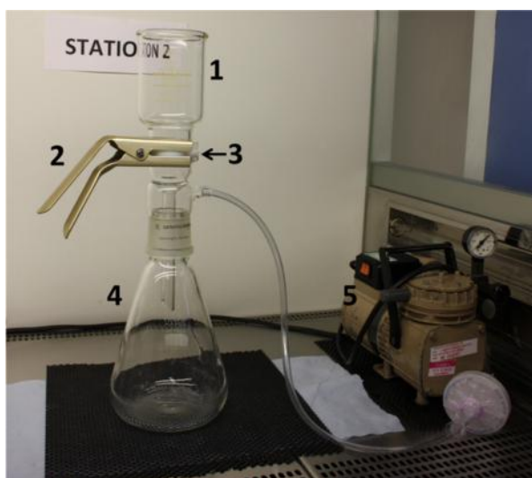
Figure 3.2 - Assembled filtration unit for isolating nanoscale and micron sized fraction of orthopaedic powder. 1 – Glass reservoir. 2 – Clamp. 3 – Filter membrane and polymer filter support. 4 – Collection flask. 5 – Vacuum pump.
