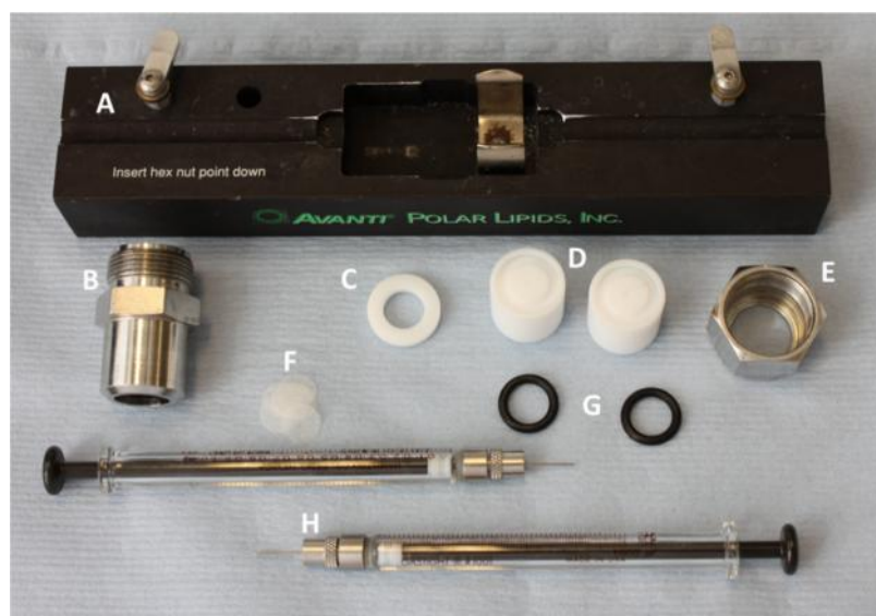
Figure 2.6 – Components of the vesicle extruder. A – Extruder holder. B – Large extruder outer casing. C – Teflon bearing. D – Internal membrane supports. E – Small extruder outer casing. F – Filter supports. G – O-rings. H – Glass syringes.
