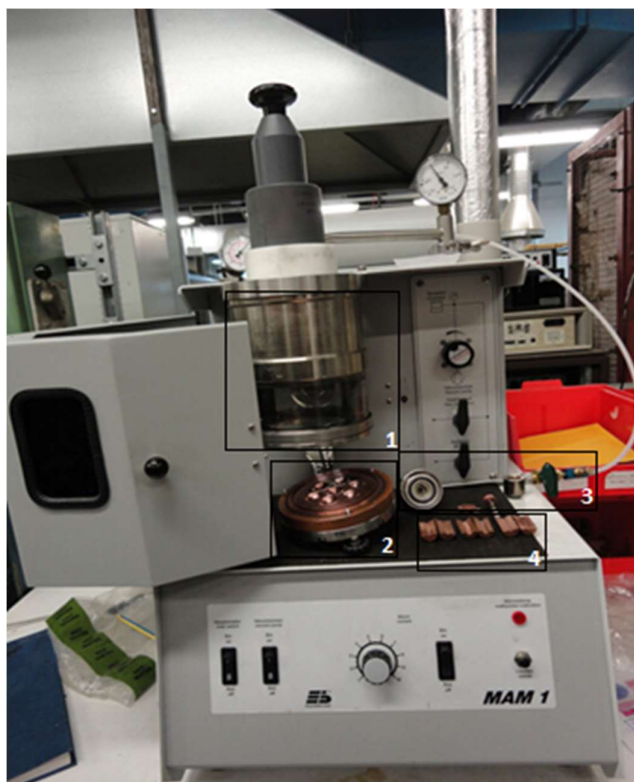
Figure 12. Figure showing the Edmund Buhler MAM 1 arc-melter.
