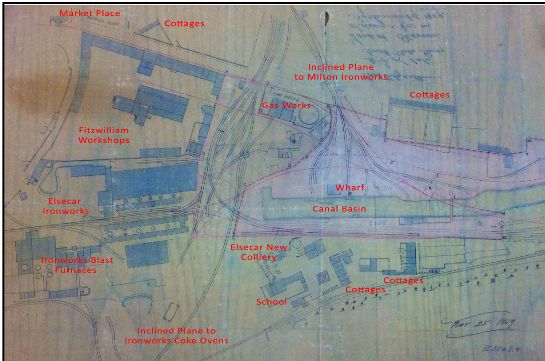
Figure 5.8 Map of Elsecar, 1859 (not to scale). The map shows details of the juxtaposition of domestic and industrial space and depicts a palimpsest of structures that date from the period 1795-1858 (modern annotations by the author are in red). Compare with the zoned and ordered plan of Saltaire (Figure 5.7). The map is orientated with East to the top of the page. Source: Barnsley Archives NBC 460A.
