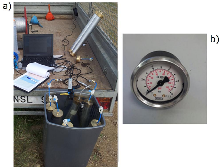
Figure 3.24 Desorption cylinders (a) and bourdon gauge (b).
