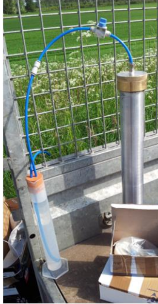
Figure 3.25 Water displacement measurement method.
