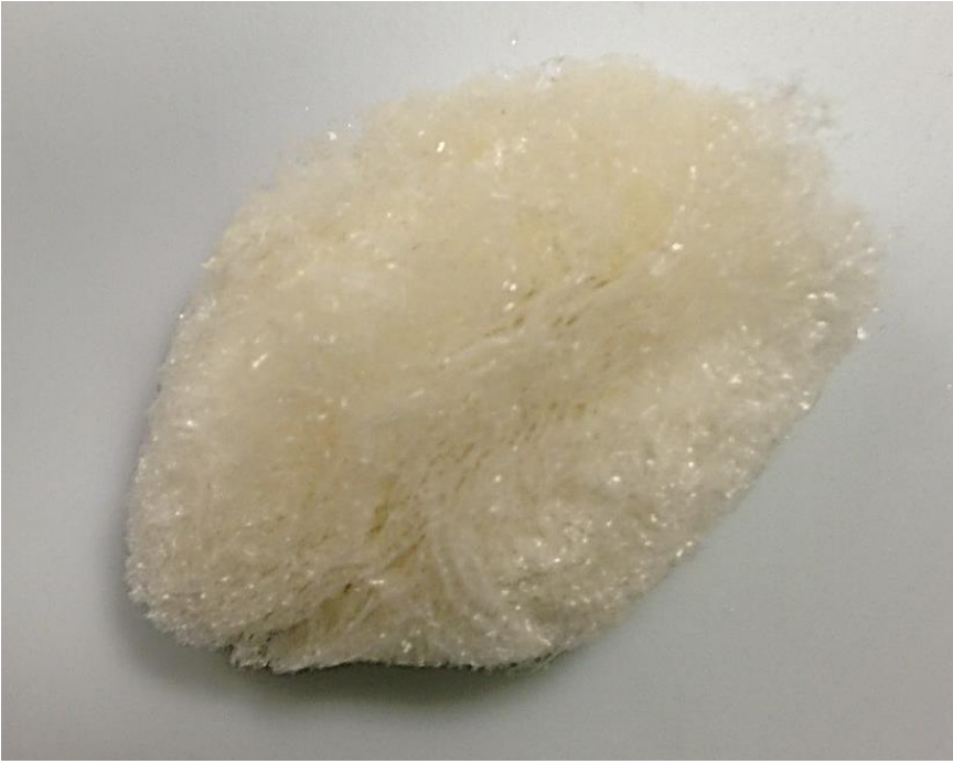
Figure 4.1: Fucoidan which has been extracted via the conventional method and freeze dried for analysis.
