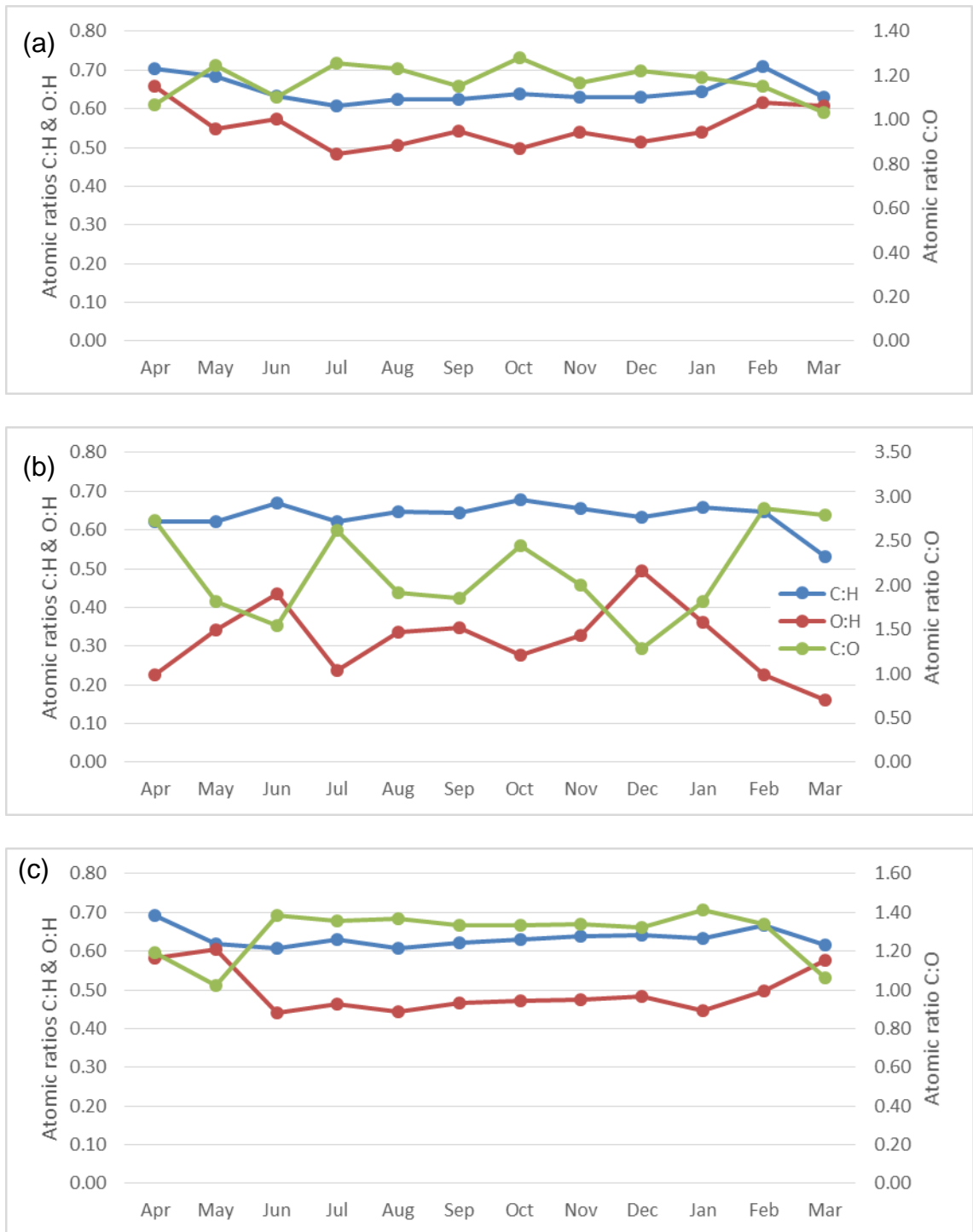
Figure 3.3: Atomic ratios calculated from CHNS on a d.a.f. basis analysis for (a) FS, (b) FV and (c) AN.
