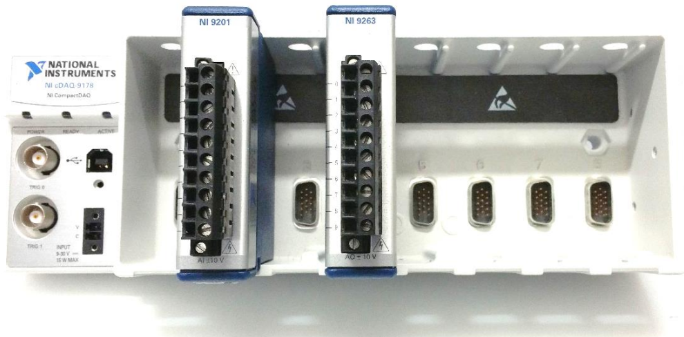
Figure 3.10: Chassis NI cDAQ 9178 with one analogue input module NI 9201 for acquiring load cell data. And one analogue output module NI 9263 for sending the signal to the motor driver for controlling the electrical pulse applied to the solenoid.
