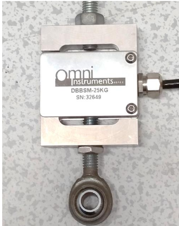
Figure 3.8: S-Beam bidirectional load cell used to measure the magnetic adhesive force generated by the EPM device. The load cell measures the pull exerted by the attached EPM device.
