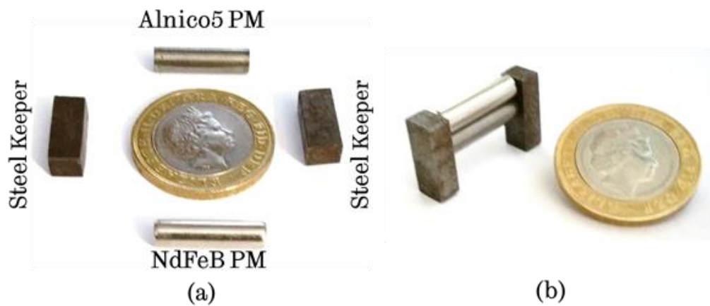
Figure 3.6: Components of the EPM used for validation of the concept. (a) EPM components: one Alnico5 PM, one NdFeB N42 PM and two mild steel keepers. (b) Basic EPM configuration: NdFeB PM is placed on top of the Alnico PM, both PMs are topped with a keeper at each magnetic poles. (Coin shown for scale purposes).
