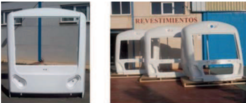
Figure 3.2: Application of the CGRP composite under analysis. Image provided by UCLM.
