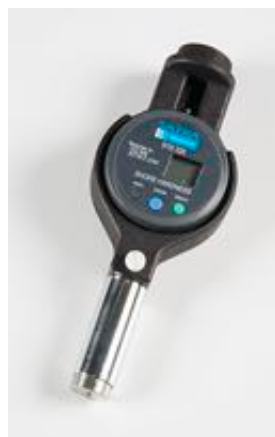
Figure 3.11 SATRA STD 226 Digital durometer
