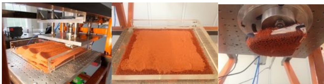
Figure 5.14 Left: The laboratory based traction rig; Centre: ACC surface prepared and mounted; Right: Shoe sample attached.
