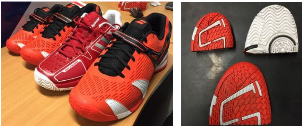
Figure 3.20 Left: Tennis shoes tested adidas Barricade 7 and Babolat 4 propulse (small, medium and large). Right: Examples of shoe outsoles.
