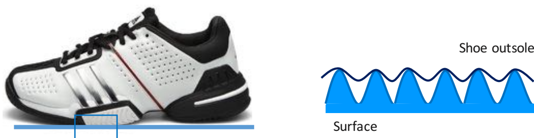
Figure 2.14 Left: Shoe-surface interface; right: Representation of the interaction between their asperities.
