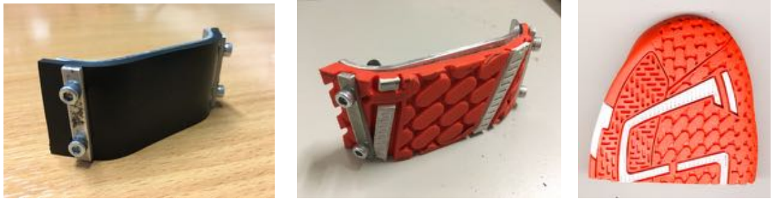
Figure 7.18 The three test rubber utilised, from left: smooth rubber, Babolat pimples and the Babolat shoe.
