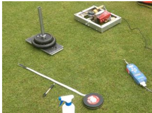
Figure 5.1 The Crab III (top right) and the bespoke sled (left) devices.
