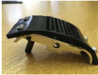
Figure 7.35 Example of uneven wear of holes sample.
