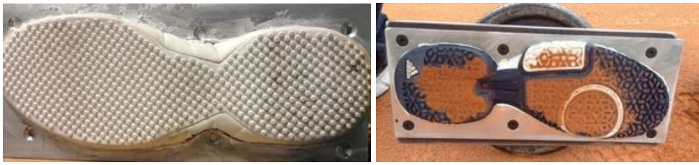
Figure 5.2 Grass and omni outsoles used with the Sled device.
