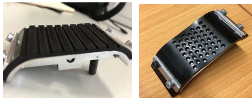
Figure 7.14 Top: Actual CNC machined test samples: Machined treads (left); Holed rubber (right).
