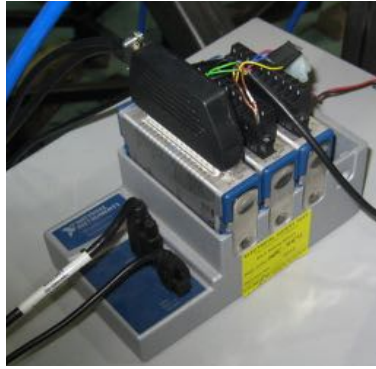
Figure 7.5 Data acquisition device with signal conditioning modules.
