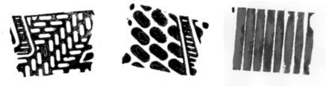
Figure 7.17 Examples of ink prints used to calculate pressures. Babolat dimples (left), Babolat pimples (centre) and machined treads sample (right).
