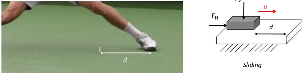
Figure A - 2 Actual (left) and schematic (right) representation of a sliding movement showing sliding displacement ( d ), vertical and horizontal forces ( F_V and F_H ) and sliding velocity ( v ).
