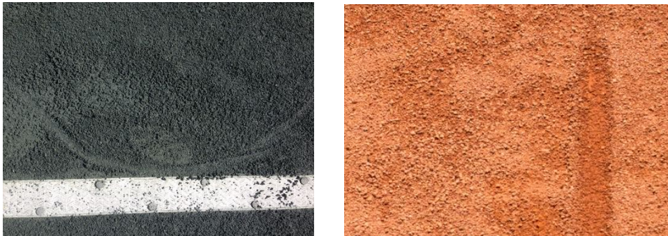
Figure 2.3 Example of the different levels of crushed brick on grey and red clay tennis courts.
