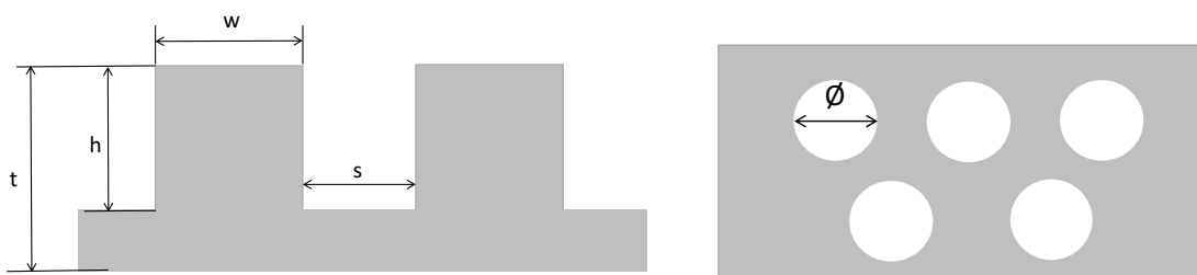
Figure 7.12 Left: representation of dimensions for total thickness ( t ), tread height ( h ), tread width ( w ) and space between treads ( s ). Right: representation of hole diameter ( \phi ).
