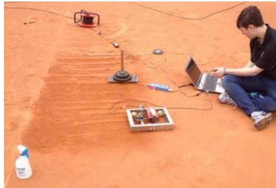
Figure 5.5 Clay testing on LTA-4 court with the sled and Crab III devices.
