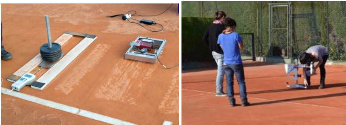
Figure 5.13 Left: The bespoke sled and The Crab III; Right: The pendulum device.
