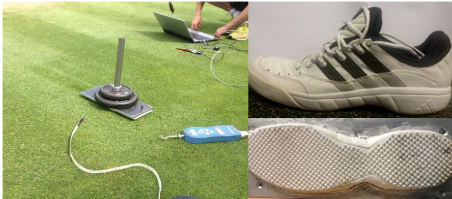
Figure 3.5 The sled test device with a grass outsole attached.
