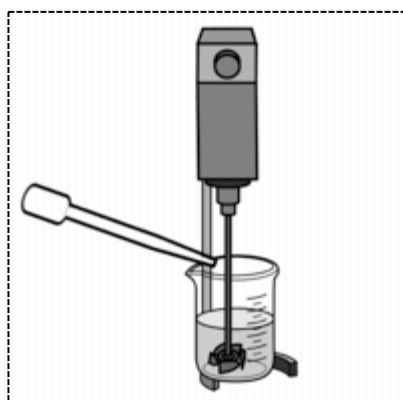
Figure 18: Schematic representation of polyHIPE preparation set-up using a high shear stirrer (1000 rpm).
