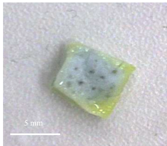
Figure 34: PLA/HA (20% w/w) structure recreated from design 3 via DMD stereolithography [Images courtesy of C.Gabbott].
