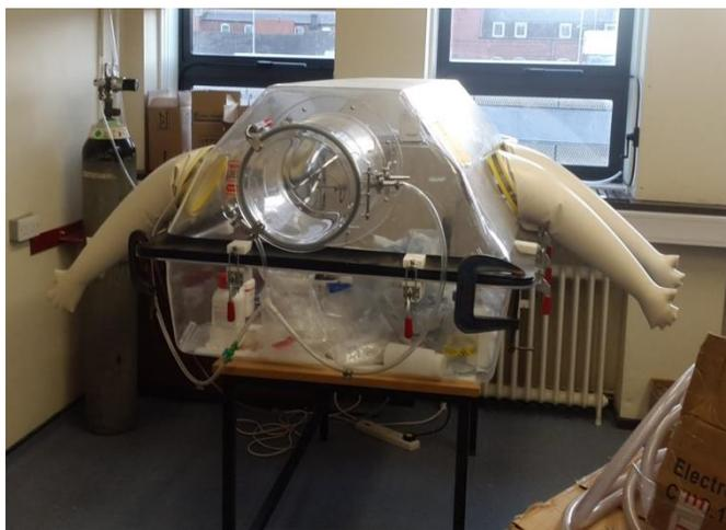
**Figure 3.1.** Image of glovebox with  $N_2$  cylinder used for high-pH dissolution experiments.
