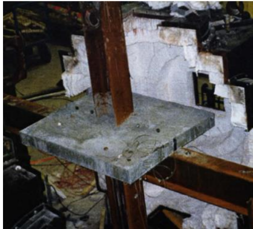
Figure 4.16: Flexible end plate composite connection detail – Group 4 [35]
