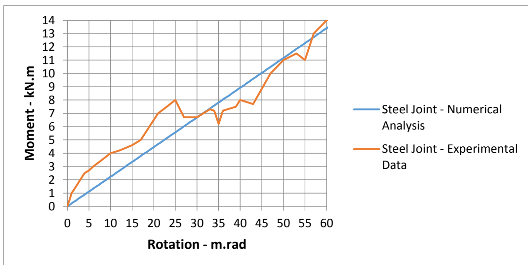
Figure 4.8: Moment-rotation curve of S2 – comparison of numerical analysis with experimental data
