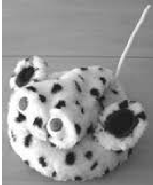
Figure 5.1. Modified iRobot Roomba as used in Jones et al. (2008). Unit shown is that for Condition 1: canid mechanisms included a tail that could be raised, lowered and wagged; ears that covered wireless speakers which emitted barking and whining sounds; and eyes that moved. A spotty fur covering was used to create a zoomorphic appearance.
