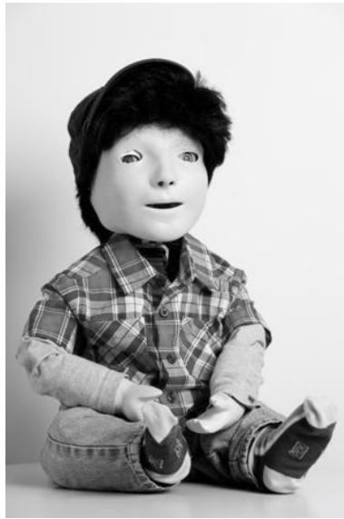
Figure 2.1. KASPAR is a minimally-expressive humanoid robot designed as a therapeutic ‘toy’ for children with ASD. It was designed by the University of Hertfordshire’s Adaptive Systems Research Group.
