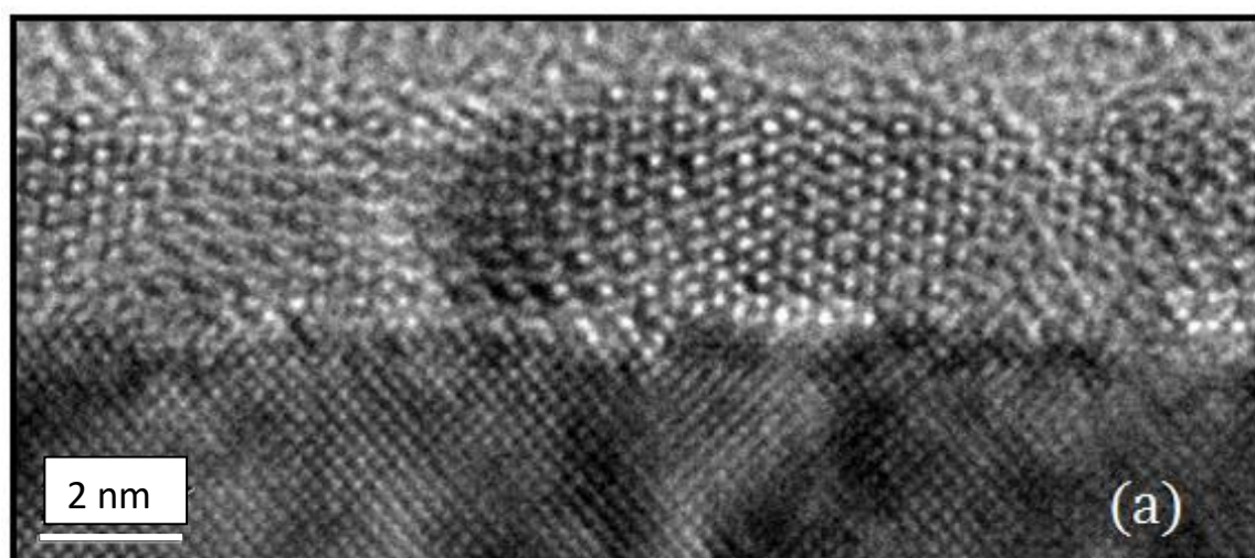
Figure 6.9: (110) direction HRTEM of (a) 9 minutes post-oxidized sample, showing Fe (100), Fe 3 O 4 (110) and substrate. Interface transition takes place over ~5 monolayers.
