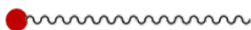
Figure 6: The structure of a surfactant with the hydrophilic head group (shown in red) and the hydrophobic tail (shown in black) 60
