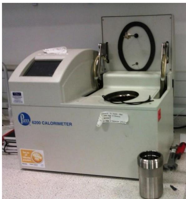
Figure 5-13: Parr 6200 Calorimeter used to determine gross calorific value
