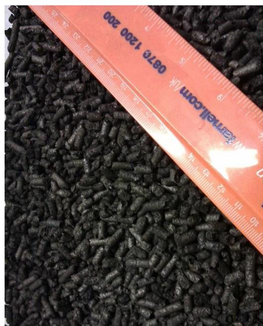
Figure 12-3: (a) The pyrolysis unit, showing the feed trough and the end cap adjacent, (b) a sample of wood pellets after pyrolysis
