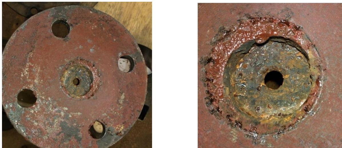
Figure 5-4: The orifice plate removed from the experimental rig, showing damage from corrosion
