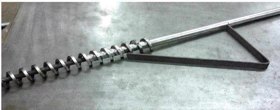
Figure 5-5: The original screw shaft from the screw feeder, showing a reduction in shaft diameter at the lower end, leaving a gap between the shaft and the screw thread
