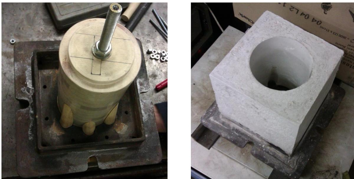
Figure 5-19: (a) wooden mould used for quarl construction, (b) the completed replica quarl
