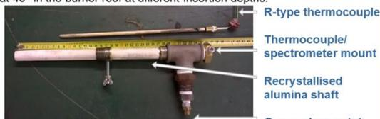
Fig 3: Photograph of burner probe
