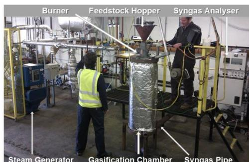
Fig 2: Photograph of gasifier rig
