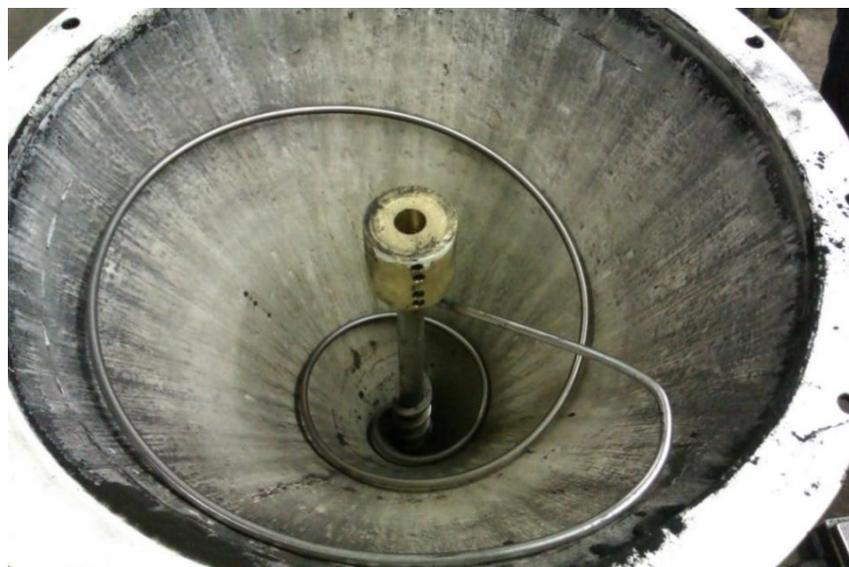
Figure 5-6: Modified helical agitator extending to the hopper wall
