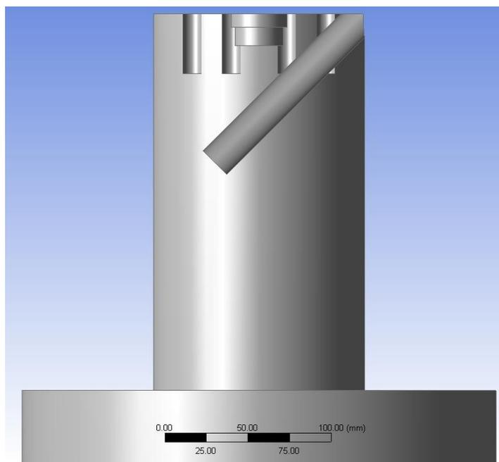
Figure 4-19: Representation of suction pyrometer inserted into quarl space
