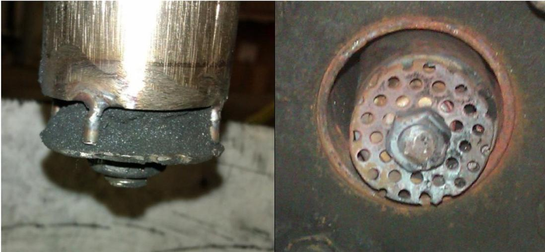
Figure 5-9: Distributor attached to bottom of screw shaft to avoid coal agglomeration; (a) side view, (b) from below
