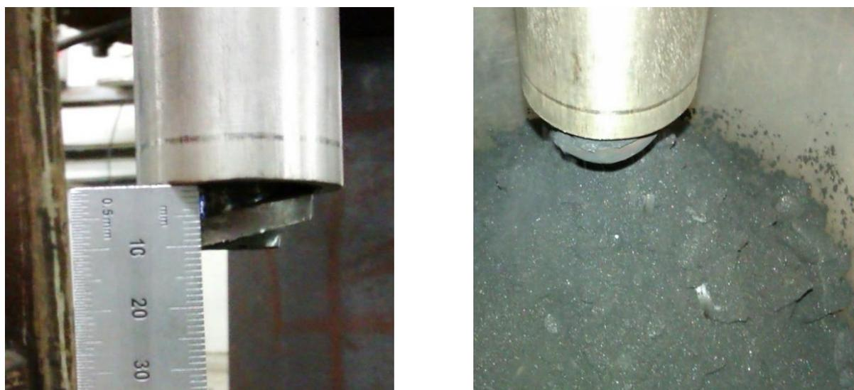
Figure 5-8: Screw feeder outlet, (a) the protrusion from the pipe, (b) agglomeration of coal through the screw feeder
