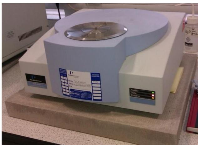
Figure 5-12: Perkin Elmer TGA 4000 used for proximate analysis
