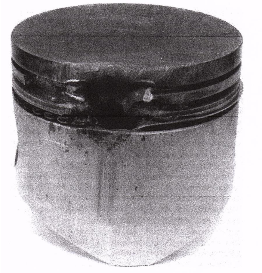
Figure 1.2 Knock damage sustained by an engine piston, from Bradley and Morley (1997)
