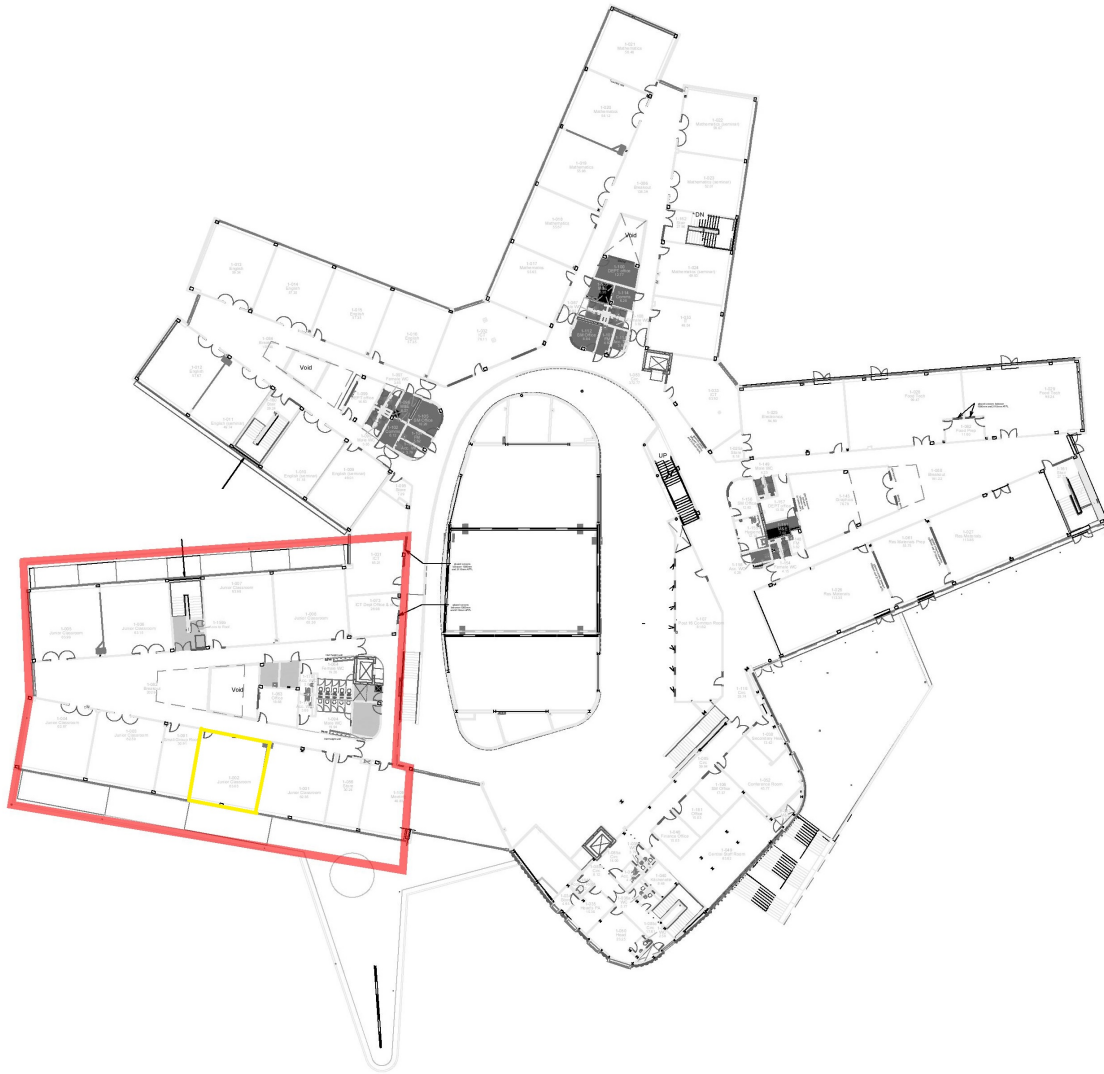
Figure 5.1: Floor plan of the school building, the red area represents the wing modelled with the zone studied bordered in yellow.
